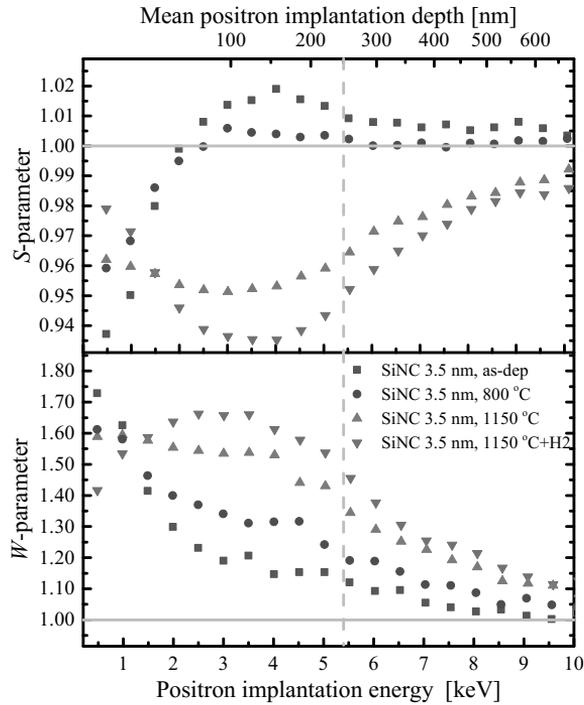
**Figure 4.3.** Normalized  $S$ - and  $W$ -parameters as a function of positron implantation energy. Full lines represent the corresponding parameters for bulk Si. The dashed line denotes the interface between the deposited layer and the substrate.
