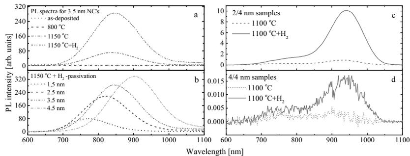
**Figure 4.2.** Photoluminescence intensities as a function of wavelength. Shown on the left are PL spectra from 3.5 nm SiNC samples after each production step (panel a) and from passivated samples having varying nanocrystal sizes (panel b). On the right PL spectra from RF sputtered samples with 2 nm (panel c) and 4 nm (panel d) Si layer.
