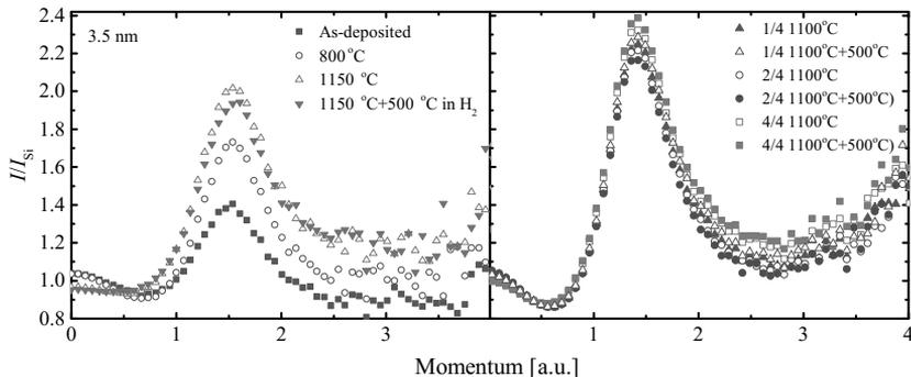
**Figure 4.5.** On the left ratio spectra from 3.5 nm sample measured after various production steps. Positrons were implanted with the energy of 3.5 keV. Dashed lines denotes the window used in determining the  $W$ -parameter value in the analysis. On the right ratio spectra from 1/4, 2/4 and 4/4 samples grown RF sputtering. Positrons were implanted with the energy of 2.0 keV. A defect free bulk Si sample was used as a reference. All measurements were performed at room temperature.
