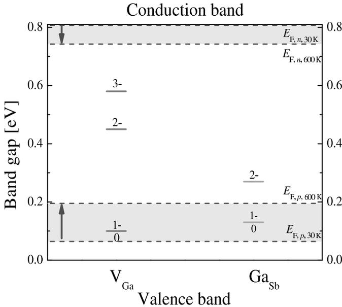
**Figure 7.3.** The GaSb band gap with the charge transition levels of  $V_{\text{Ga}}$  and  $\text{Ga}_{\text{Sb}}$  after Virkkala *et al.* [66]. The Fermi-level positions at 30 K and at 600 K in  $p$ - and  $n$ -type GaSb are represented with purple dashed lines. Yellow color indicate the area covered by the Fermi-level when the temperature is increased or decreased. The arrows indicate the direction of the Fermi-level movement when the temperature is increased.
