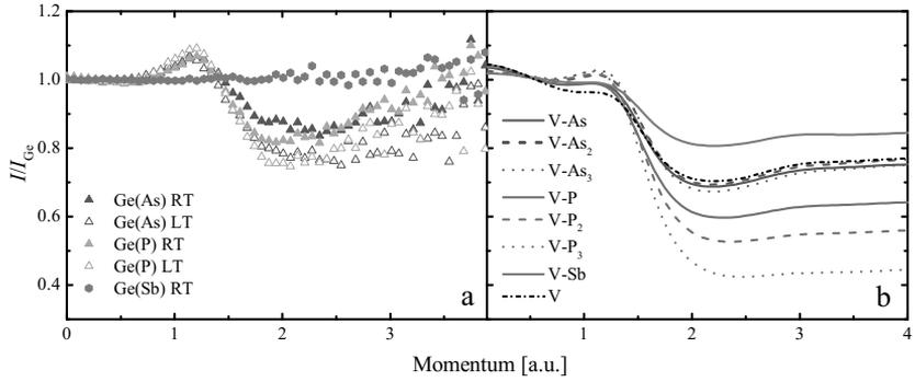
**Figure 6.2.** Experimental (panel a) and calculated (panel b) positron-electron momentum distribution ratios for Ge(As), Ge(P) and Ge(Sb).
