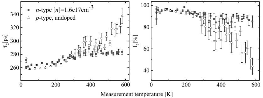
**Figure 7.1.** Lifetimes (left) and intensities (right) as a function of temperature obtained from the two-component model.
