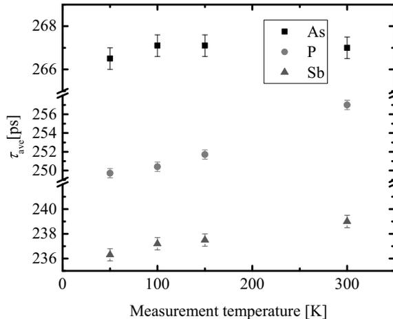
**Figure 6.1.** The average positron lifetimes in highly doped as-received Ge.
