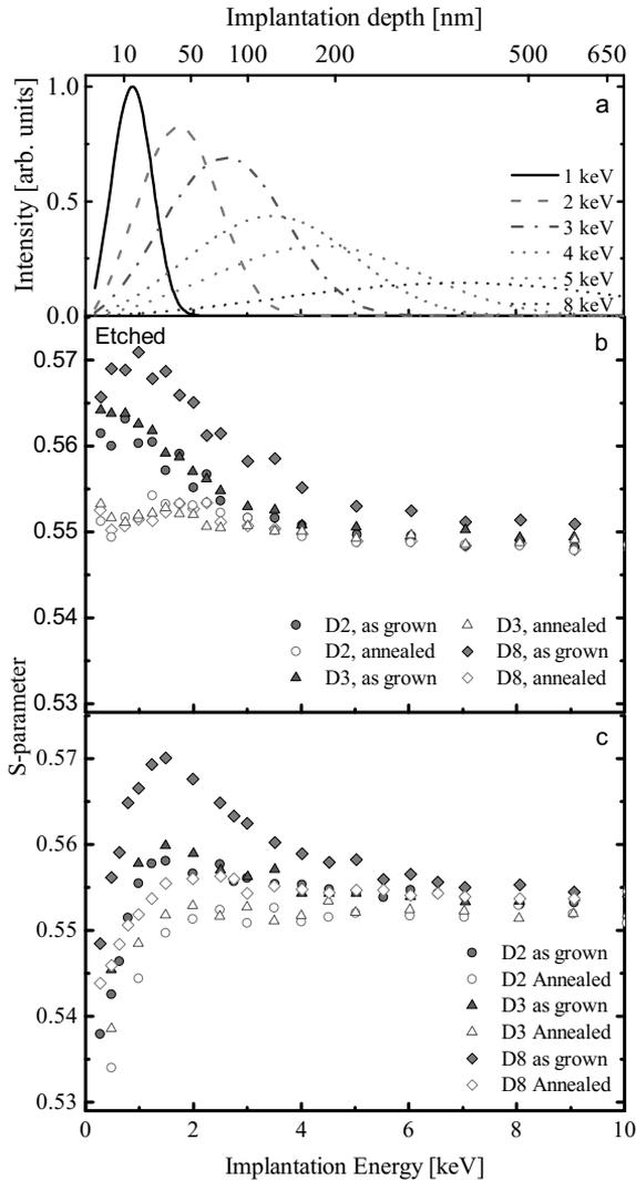
**Figure 5.1.**  $S$  parameters as a function of positron implantation energy after and before the etching (panels b and c). Panel a shows the positron implantation profiles for various energies. Values in the upper horizontal axis shows the mean implantation depth for positrons accelerated with the matching implantation energy (lower horizontal axis). The intensities of the implantation profiles are not in scale.
