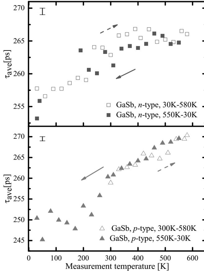
**Figure 7.2.** Positron average lifetime in *p*- and *n*-type GaSb. Open symbols indicate that the next measurement is done at a higher temperature than the preceding; the direction of the temperature change is represented by the dashed arrows. Closed symbols indicate that the next measurement is done at a lower temperature than the preceding; the direction of the temperature change is represented by the full arrows.
