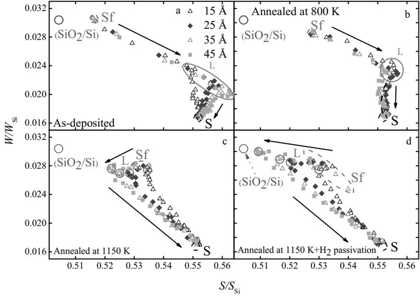
**Figure 4.4.** Normalized  $S(W)$ -plots of different SiNC sizes and and heat treatments. Arrows in the figure indicate the increasing positron implantation energy. Surface (Sf), substrate (S), layer (L) and SiO<sub>2</sub>/Si interface point [53] are denoted in the plots.
