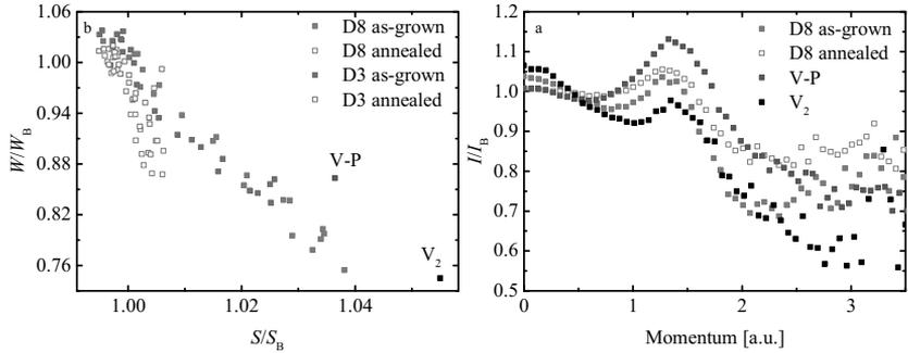
**Figure 5.2.** On the left  $(S, W)$ -plots for the samples containing 2.3% and 4.6% P are shown. On the right coincidence Doppler broadening ratio curves for the annealed and as-grown sample with 4.6% P are presented. Included are also results for the  $E$ -center (V-P) [17] and the divacancy in Si [56, 57].
