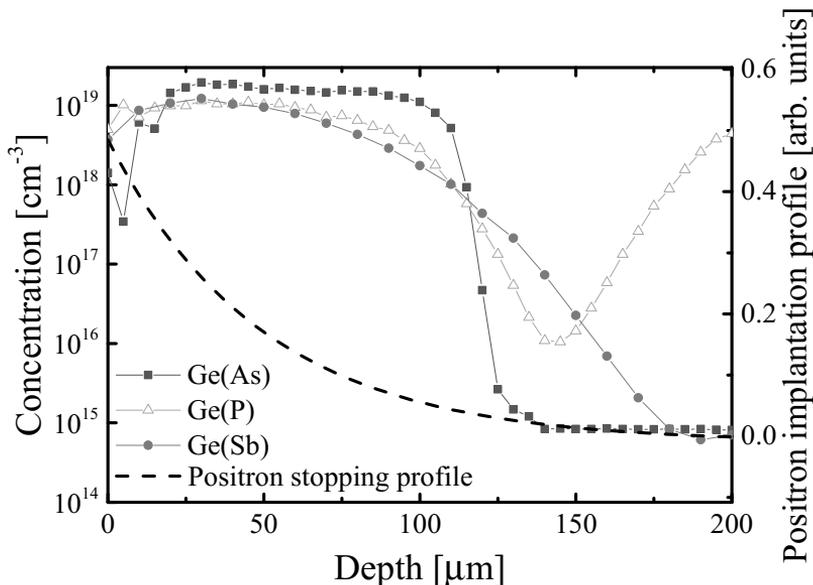
**Figure 6.3.** Dopant concentration for As, P and Sb ( $\text{cm}^{-3}$ ) in Ge obtained from the spreading resistance measurements. The calculated positron implantation profile is shown by the black dashed line in arbitrary units. The sensitivity limit for the positron annihilation is  $\sim 10^{15} \text{ cm}^{-3}$  which is set to zero (see right axis).
