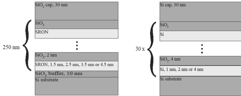
**Figure 4.1.** The structure of PECVD (left) and RF sputtered samples (right). In PECVD treated samples the layers consist of bilayers of Silicon Rich OxyNitride (SRON) and SiO<sub>2</sub> whereas in RF sputtered samples Si/SiO<sub>2</sub> layers were used.
