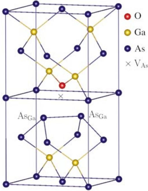
FIG. 1. Two conventional GaAs unit cells with the  $(\text{As}_{\text{Ga}})_2\text{-O}_{\text{As}}$  defect (schematically). Yellow balls denote gallium and blue balls arsenic atoms. A red ball denotes the oxygen atom, and a cross the arsenic vacancy ( $V_{\text{As}}$ ). The two arsenic antisites ( $\text{As}_{\text{Ga}}$ ) are marked in the figure.
