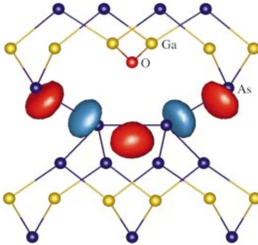
FIG. 2. A constant-value surface of the electron density of the uppermost occupied electronic state of the negative charge state of  $(\text{As}_{\text{Ga}})_2\text{-O}_{\text{As}}$ . The electron density isosurface is at half of the maximum value of  $0.03e/\text{\AA}^3$ . Yellow balls denote gallium, and blue balls arsenic atoms. A red ball denotes the oxygen atom. A red surface indicates positive wave function and a blue surface negative one.
