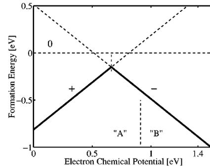
FIG. 3. Formation energy plot for the  $(\text{As}_{\text{Ga}})_2\text{-O}_{\text{As}}$  defect. The thick line indicates the charge state with the lowest energy. The energy of the metastable neutral charge state is taken as the reference energy. The experimental band-gap value of 1.53 eV is used to give the upper limit for the electron chemical potential. "A" and "B" denote the two experimentally observed (Refs. 3 and 6) stable states separated by an ionization level.
