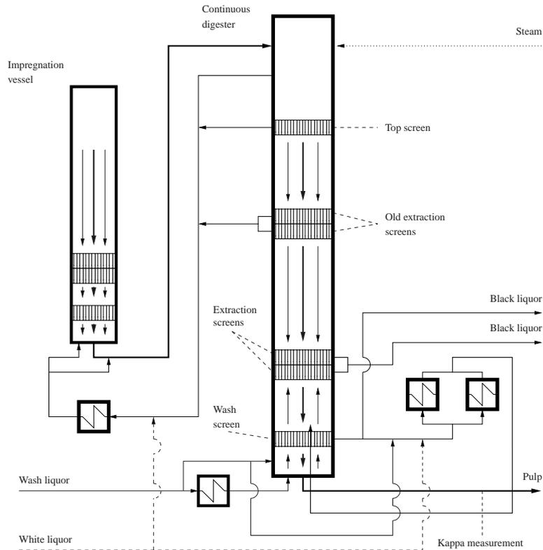
**Figure 5. The continuous digester and the impregnation vessel. The cooking and wash liquor flows are marked by thin lines and the chip flow by the thick line. The four square-shaped symbols are heat exchangers.**
