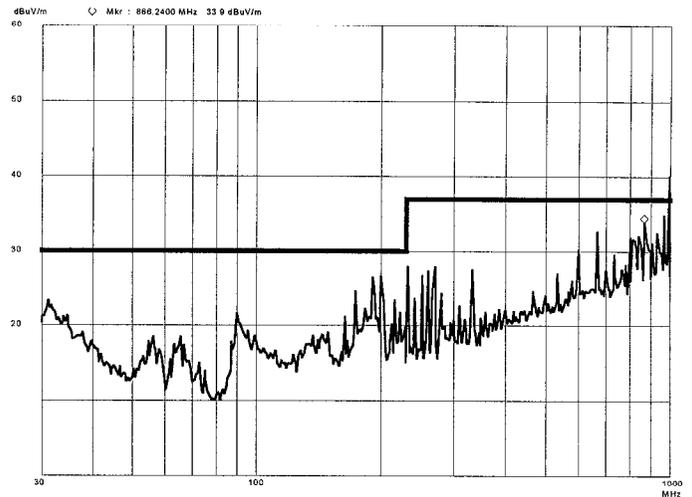
**Figure 2. Radiated emissions from PC CPU with a closed enclosure. [6]**
