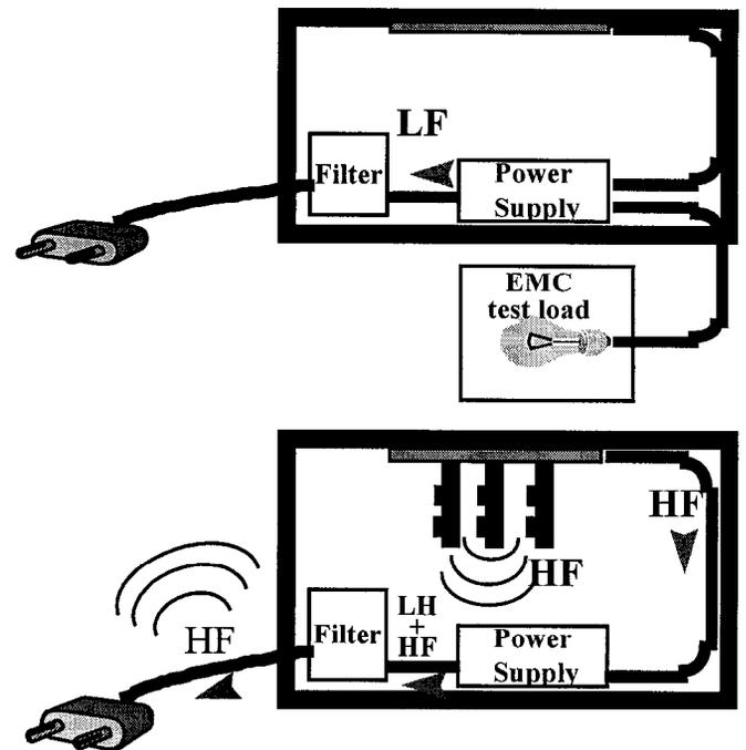
Figure 1. The effect of EMC test load
