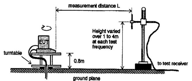
Figure 5. The setup for the radiated emission test.
