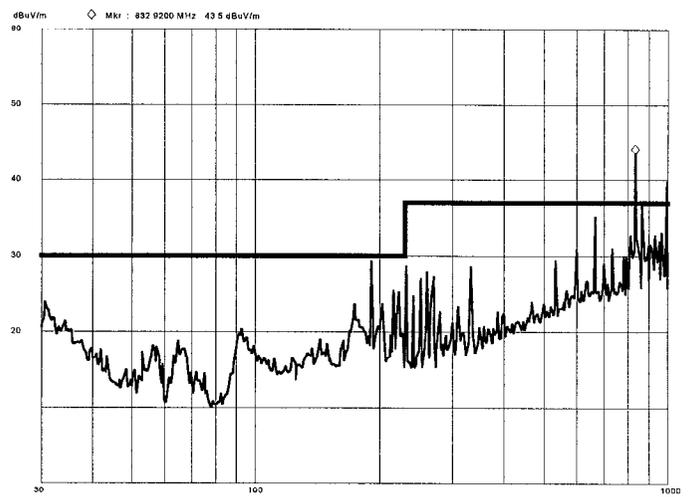
**Figure 3. Radiated emissions from PC CPU with a thin enclosure. [6]**
