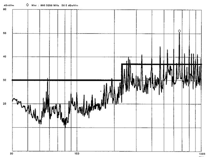
**Figure 4. Radiated emissions from PC CPU with an open enclosure [6]**
