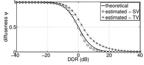
**Fig. 2.** Theoretical diffuseness curve and estimated one for a tetrahedral arrangement and ideal cardioid sensors.
