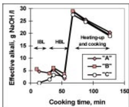
Fig. 4. Alkali profiles during SuperBatch simulations.
