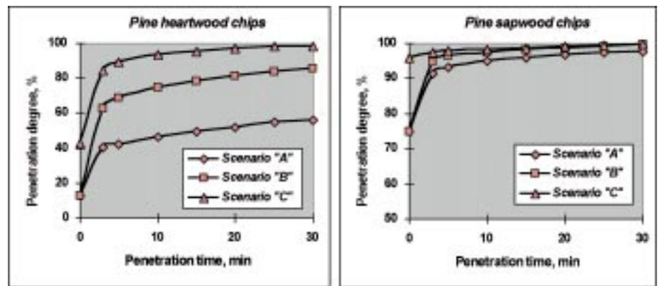
Fig. 3. Black liquor penetration into pine chips.
