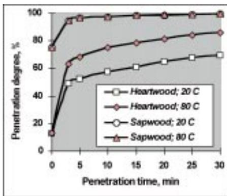
**Fig. 8.** Effect of temperature on black liquor penetration into pine chips; over-pressure - 9 bar.
