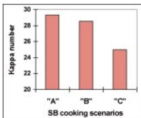
Fig. 6. Kappa number of SuperBatch pulps.
