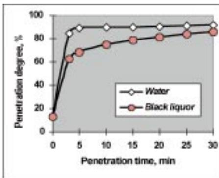
**Fig. 9.** Black liquor vs. water; penetration scenario "B".
