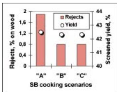
Fig. 5. Rejects and yields from the SuperBatch cooks.
