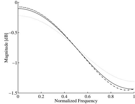
Figure 7: The desired magnitude response (dash-dotted) obtained from the truncated polynomial and the magnitude responses of the fitted IIR filters. The filter orders are one,two, and six, and they are plotted with dotted, solid, and dashed lines respectively.
