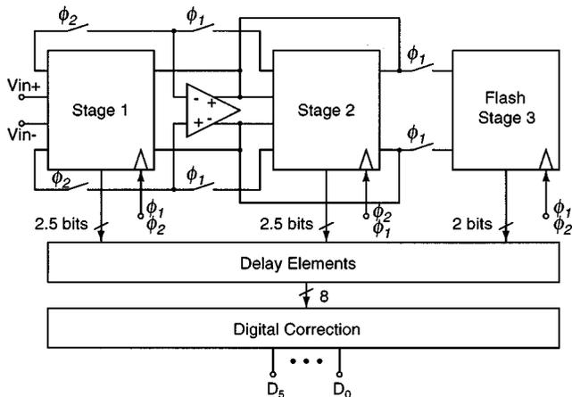
Fig. 5. A/D converter block diagram.
