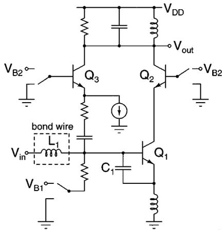
Fig. 2. Single branch of the LNA in high gain mode.
