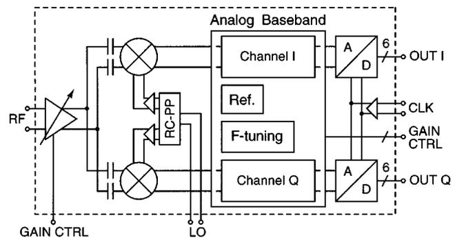
Fig. 1. Receiver block diagram.
