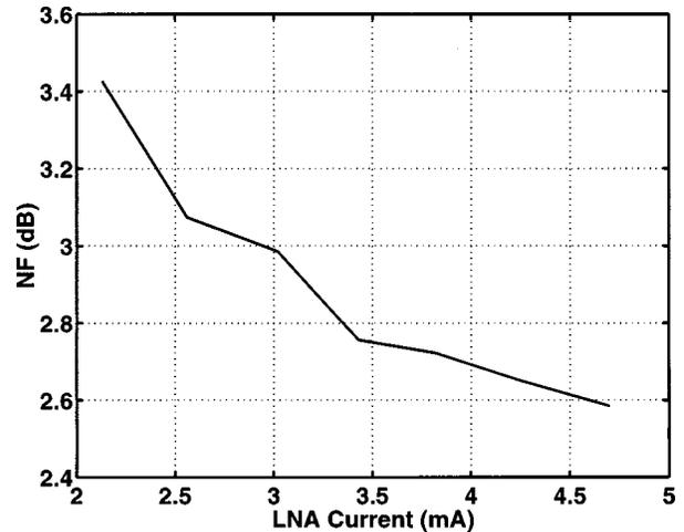
Fig. 7. Receiver NF as a function of the LNA quiescent current.
