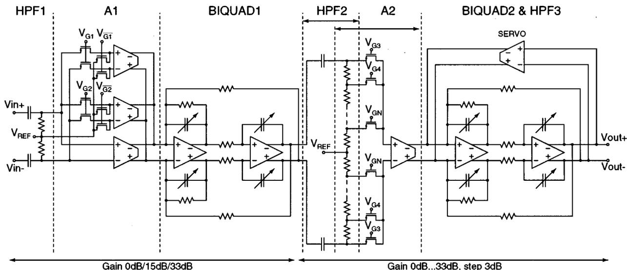
Fig. 4. One signal channel of the analog baseband circuit.
