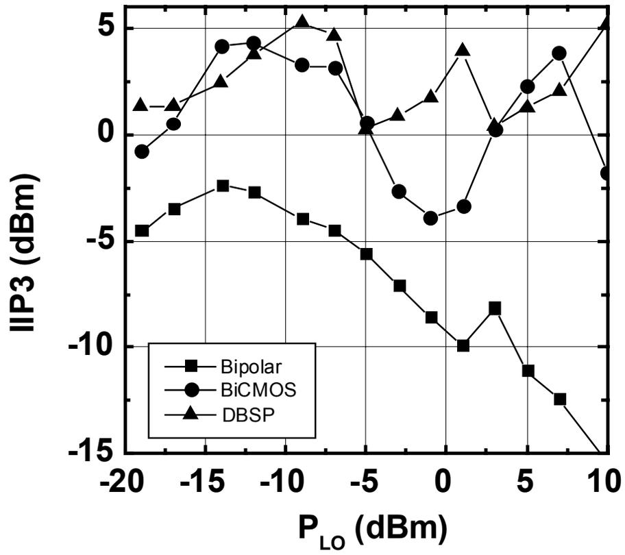
Fig. 7. Measured IIP3 vs. LO power.
