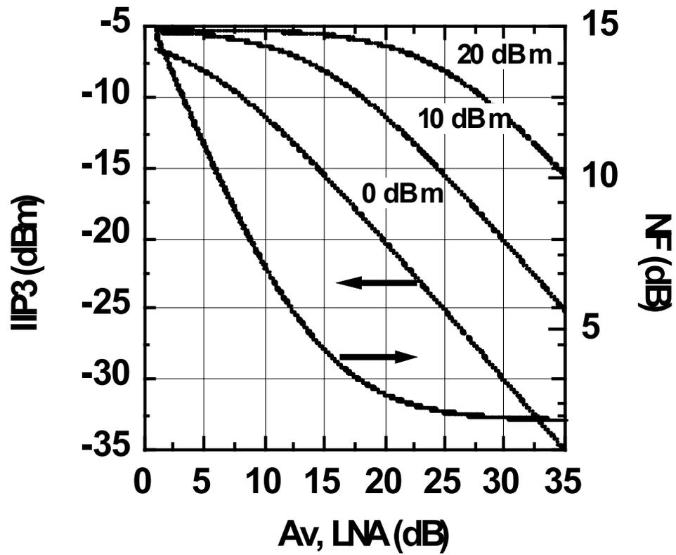
Fig. 2. IIP3 and NF of the front-end for three different mixer IIP3 values. The DSB noise figure of the mixer is assumed to be 10 dB and the IIP3 and NF of the LNA are  $-5$  dBm and 2 dB, respectively.
