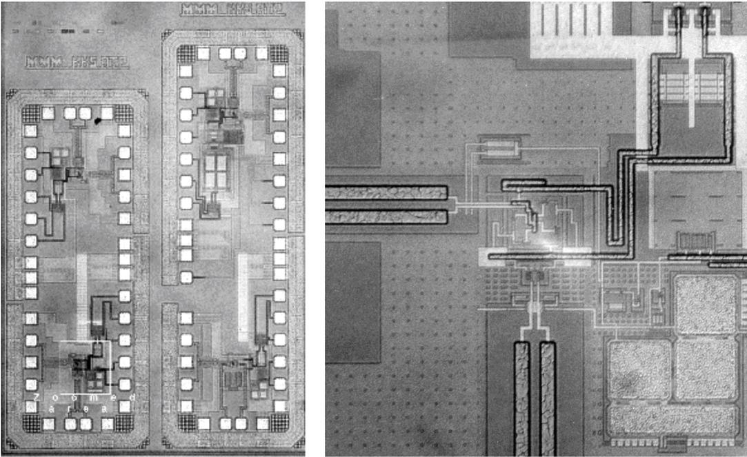
Fig. 4. Microphotograph of the test chip and bipolar mixer core.
