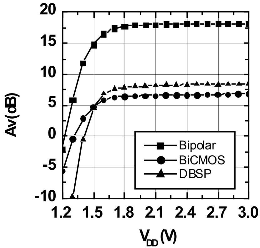
Fig. 8. Conversion gain vs. supply voltage for different mixers.
