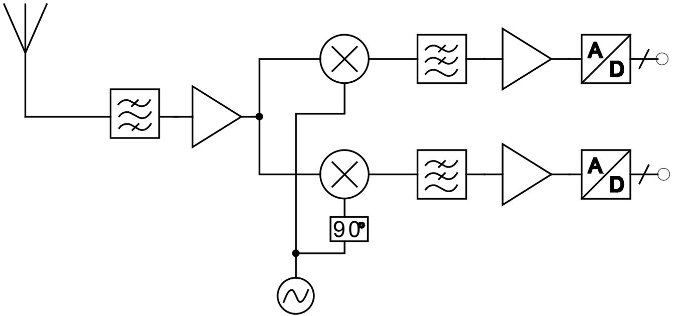
Fig. 1. Block diagram of direct conversion receiver.
