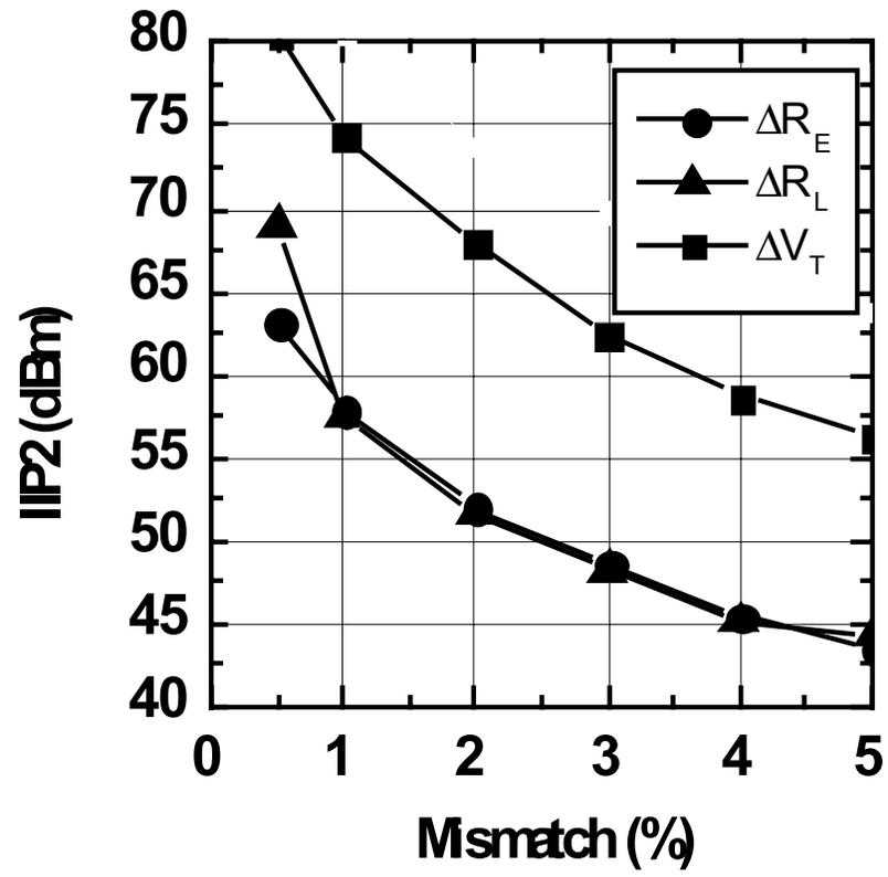
Fig. 10. IIP2 vs. three different mismatches in BiCMOS mixer.
