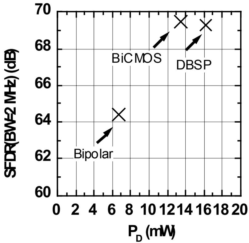
Fig. 11. Spurious free dynamic range of each mixer for 2 MHz bandwidth vs. power dissipation.
