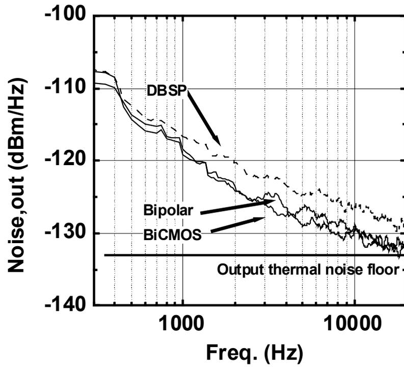
Fig. 5. Measured flicker noise performances of different mixers.
