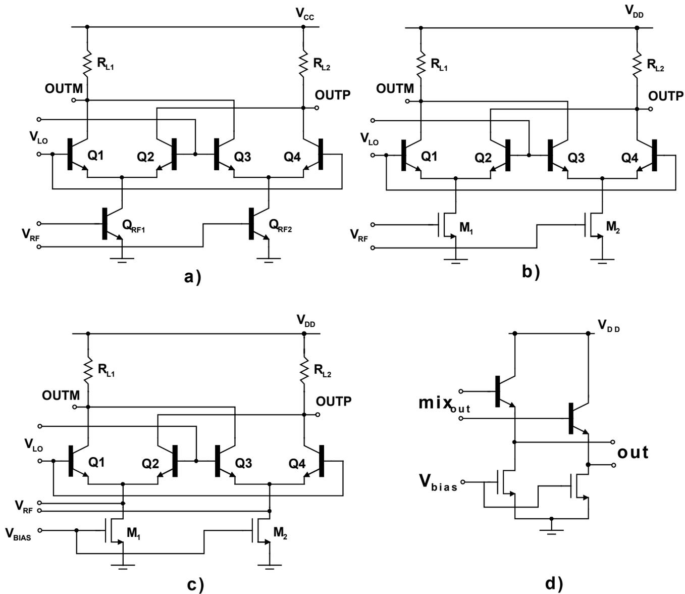
Fig. 3. Implemented a) bipolar, b) BiCMOS, c) DBSP mixer, d) output buffer.
