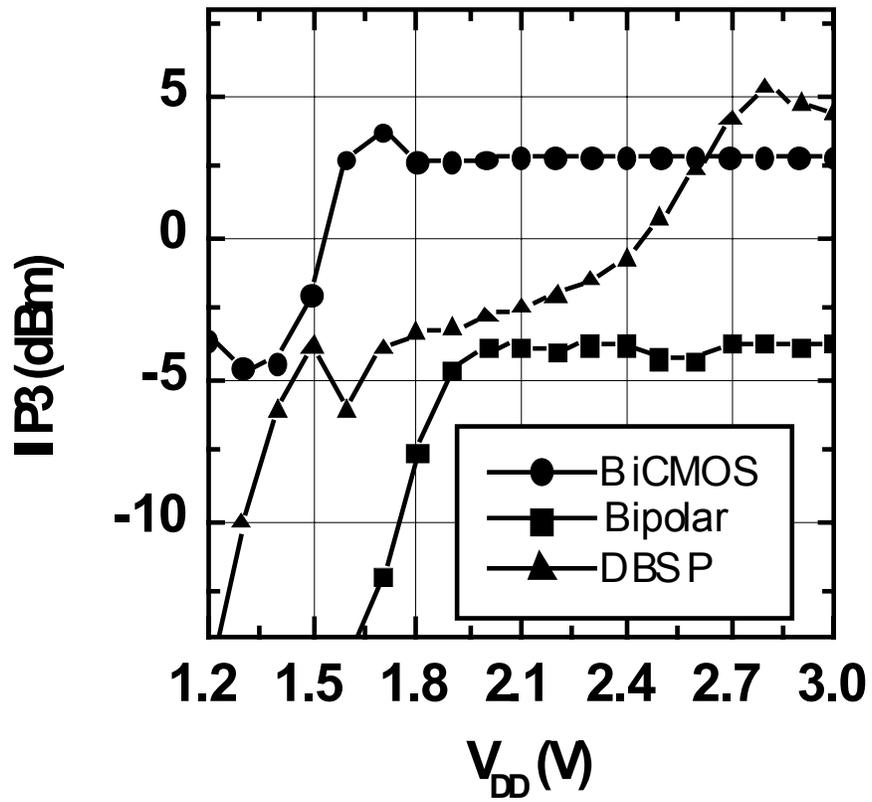
Fig. 9. IIP3 vs. supply voltage for different mixers.
