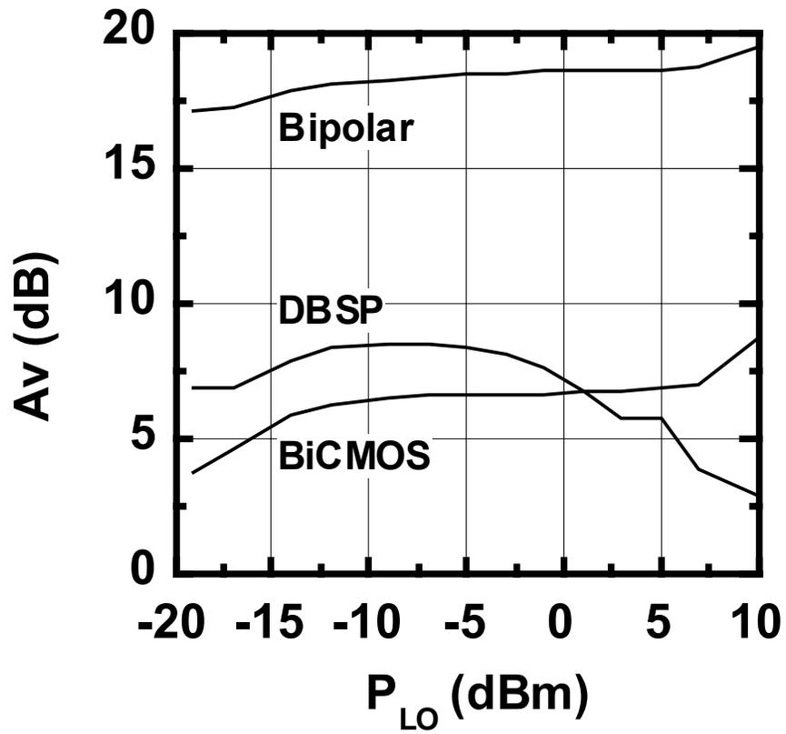
Fig. 6. Voltage gain vs. LO power for different mixers.
