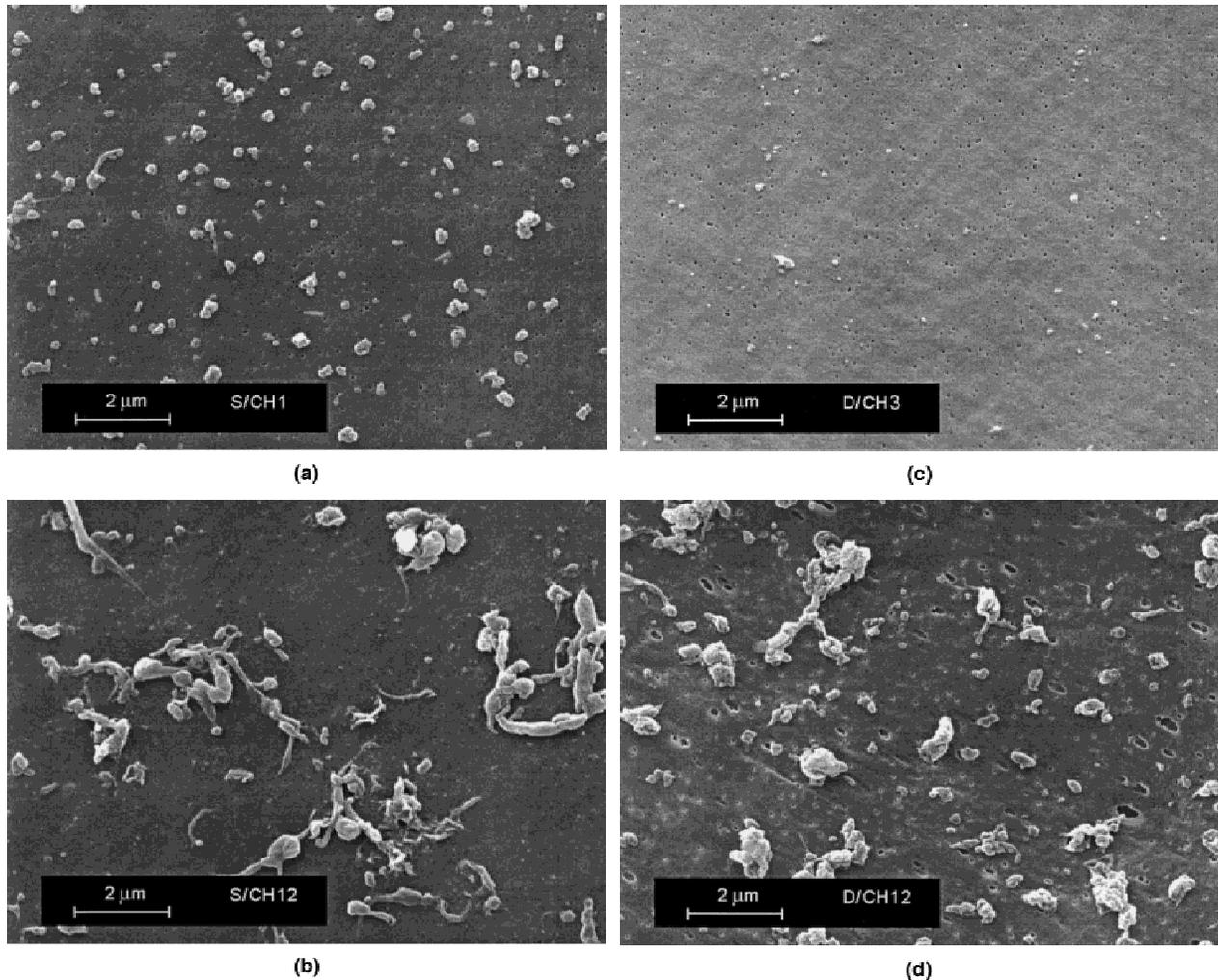
**Figure 5.** Scanning electron micrographs from 0.05- $\mu\text{m}$  pore size Nucleopore membranes, through which the digested samples of serum lubricant were filtered, showing polyethylene wear particles. (a) Conventional polyethylene, counterface  $R_a = 0.022 \mu\text{m}$ ; (b) conventional polyethylene, counterface  $R_a = 0.24 \mu\text{m}$ ; (c) crosslinked polyethylene, counterface  $R_a = 0.023 \mu\text{m}$ ; (d) crosslinked polyethylene, counterface  $R_a = 0.22 \mu\text{m}$ .
