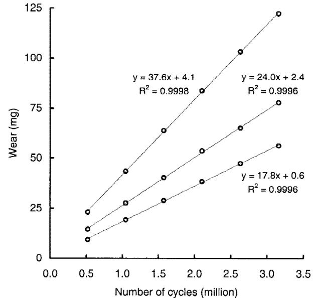
**Figure 2.** Examples of variation of polyethylene wear with number of cycles, illustrating the determination of wear rate. Conventional polyethylene pins against the three roughest disks.
