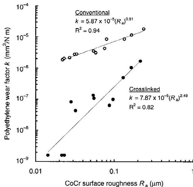
Figure 3. Variation of polyethylene wear factor with counterface surface roughness.
