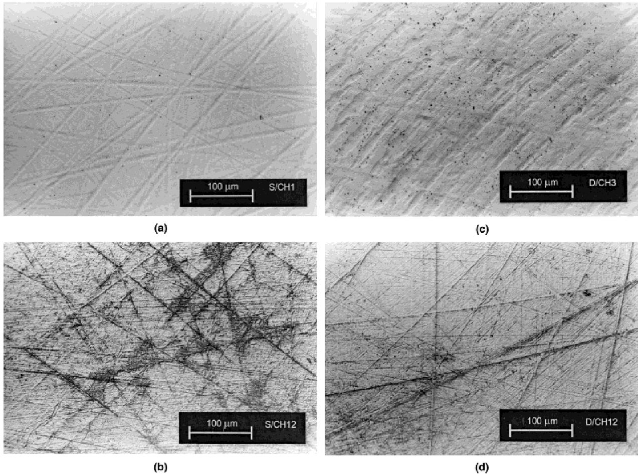
**Figure 4.** Optical micrographs from polyethylene wear faces after the tests. (a) Conventional polyethylene, counterface  $R_a = 0.022 \mu\text{m}$ ; (b) conventional polyethylene, counterface  $R_a = 0.24 \mu\text{m}$ ; (c) crosslinked polyethylene, counterface  $R_a = 0.023 \mu\text{m}$ ; (d) crosslinked polyethylene, counterface  $R_a = 0.22 \mu\text{m}$ . Note the remains of machining grooves in (c).
