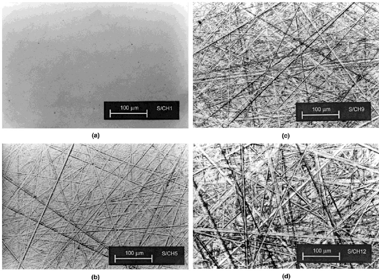
**Figure 1.** Optical micrographs from CoCr disks. (a) Polished,  $R_a = 0.022 \mu\text{m}$ ; (b) roughened,  $R_a = 0.033 \mu\text{m}$ ; (c) roughened,  $R_a = 0.080 \mu\text{m}$ ; (d) roughened,  $R_a = 0.24 \mu\text{m}$ .
