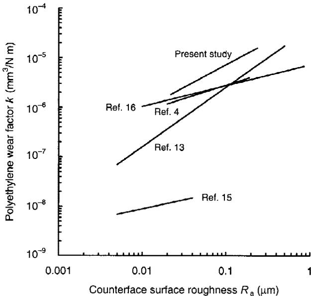
Figure 6. Present  $k$  versus  $R_a$  power relationship for conventional polyethylene compared with those found from the literature.
