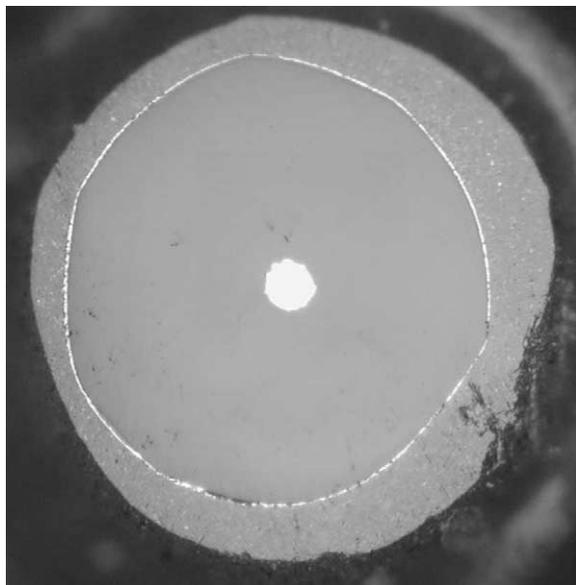
Fig. 3. A photograph of an RD electrode assembly. The diameter of the disk is 25  $\mu\text{m}$ .
