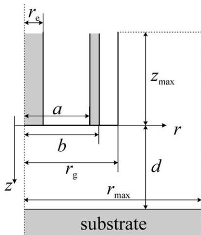
Fig. 2. Definition of the co-ordinate system and the symbols used in Section 2.
