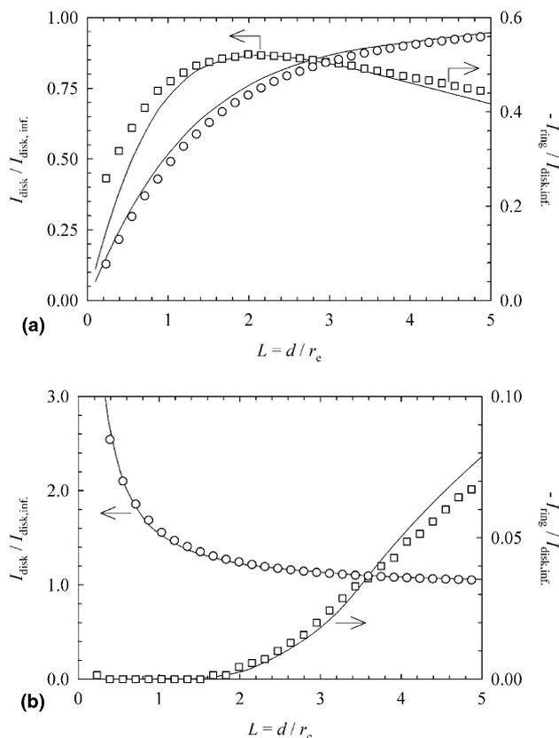
Fig. 5. Experimental approach curves (disk (O) and ring (□)) to (a) an insulating and (b) a conducting substrate.  $E_{\text{disk}} = 0.3$  V vs. Ag/AgCl,  $E_{\text{ring}} = 0$  V vs. Ag/AgCl. The disk diameter is  $25 \mu\text{m}$ . The solid lines are from numerical simulations with  $a/b = 0.995$ ,  $b/r_e = 9$ , and  $r_g/r_e = 15$ . All the curves are normalised with the limiting current at the disk far from the substrate,  $I_{\text{disk,inf}}$ .
