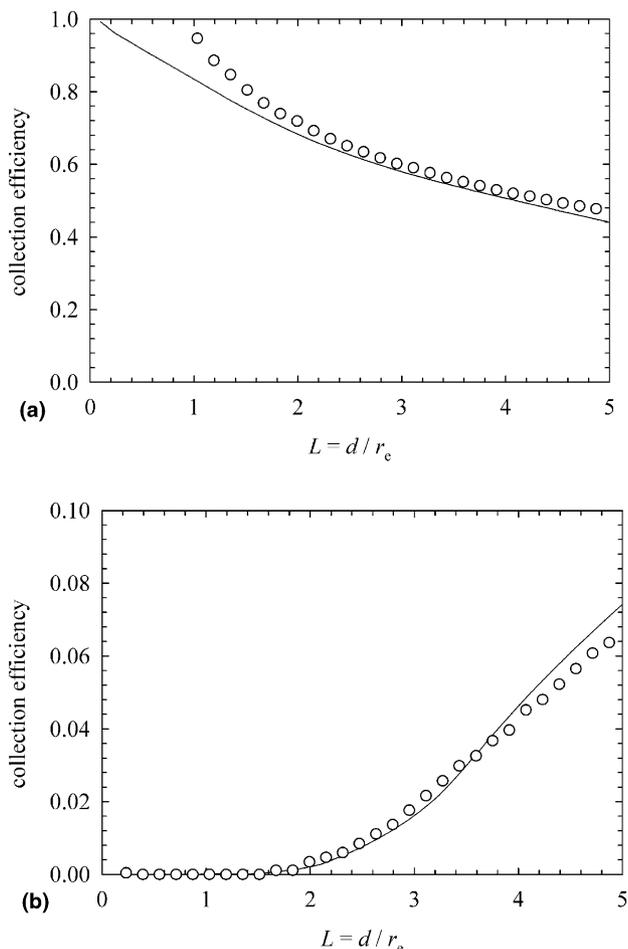
Fig. 6. The collection efficiencies ( $\eta = |I_{\text{ring}}/I_{\text{disk}}|$ ) calculated from the approach curves to an insulating (a) and conducting (b) substrate. Experimental data are represented by circles while the solid lines are from the numerical simulation.
