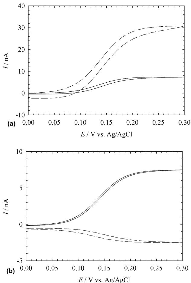
Fig. 4. (a) CVs of ferrocene methanol (2.5 mM) oxidation at the disk (—) and the ring (---). Sweep rate 25 mV/s. (b) CVs of a generation–collection experiment (disk (—), ring (---)): the potential of the disk is scanned while that of the ring is held at 0 V vs. Ag/AgCl. The disk diameter is 25  $\mu\text{m}$ .
