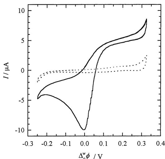
Fig. 7. Experimental cyclic voltammograms of TEA<sup>+</sup> transfer (solid line) and base electrolyte (dashed line) at the channel flow water | immobilised *o*-NPOE interface. Flow rate 525 cm<sup>3</sup> h<sup>-1</sup>. Sweep rate 2 mV s<sup>-1</sup>.
