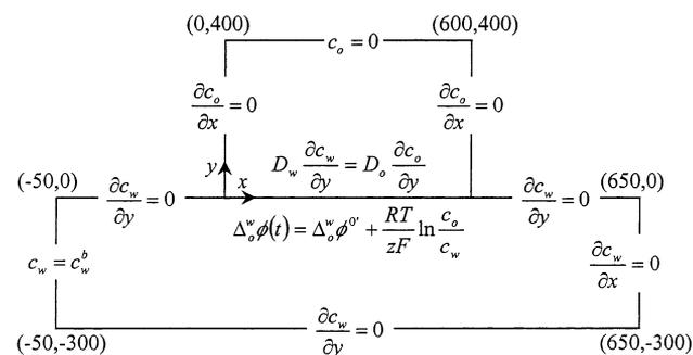
Fig. 2. Schematic presentation of the boundary conditions used. The organic phase is depicted on top of the aqueous phase. The magnitudes involved in the condition of reversible ion transfer are:  $\Delta_o^w \phi^o$  formal standard transfer potential,  $z$  charge number,  $F$  Faraday's constant,  $R$  gas constant, and  $T$  absolute temperature. The coordinates refer to values of  $(X, Y)$ .
