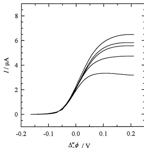
Fig. 9. Experimental linear potential sweeps of TEA<sup>+</sup> transfer at the channel flow water | immobilised *o*-NPOE interface with varying flow rate. Sweep rate 2 mV s<sup>-1</sup>. Flow rates 121, 312, 511, 711, and 906 cm<sup>3</sup> h<sup>-1</sup>.
