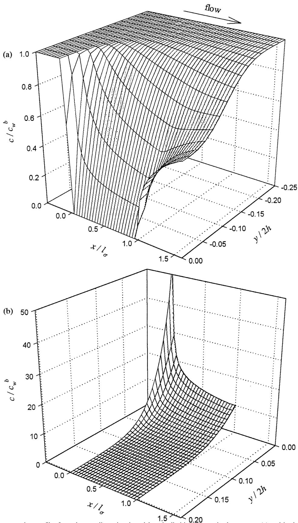
Fig. 4. Simulated concentration profiles from the two-dimensional model at the limiting current in the aqueous (a) and in the organic (b) phase. Flow rate  $100 \text{ cm}^3 \text{ h}^{-1}$ . Sweep rate  $2 \text{ mV s}^{-1}$ . Other parameter values as in Fig. 3.
