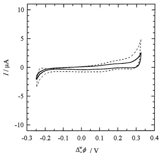
Fig. 6. Experimental base electrolyte voltammograms at the channel flow water | immobilised *o*-NPOE interface. Flow rate 520  $\text{cm}^3 \text{h}^{-1}$ . Sweep rates 2  $\text{mV s}^{-1}$  (solid line) and 10  $\text{mV s}^{-1}$  (dashed line).
