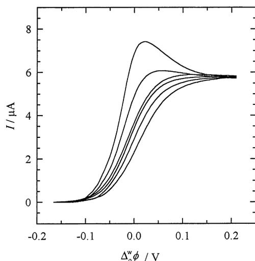
Fig. 8. Effect of the varying sweep rate on the experimental linear potential sweeps of TEA<sup>+</sup> transfer across the channel flow water | immobilised *o*-NPOE interface. Flow rate 520 cm<sup>3</sup> h<sup>-1</sup>. Sweep rates 2, 5, 8, 10, 15, and 25 mV s<sup>-1</sup>.
