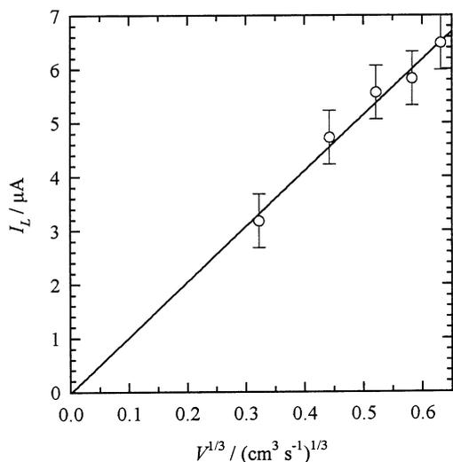
Fig. 10. The limiting current vs. the cubic root of the volume flow rate.
