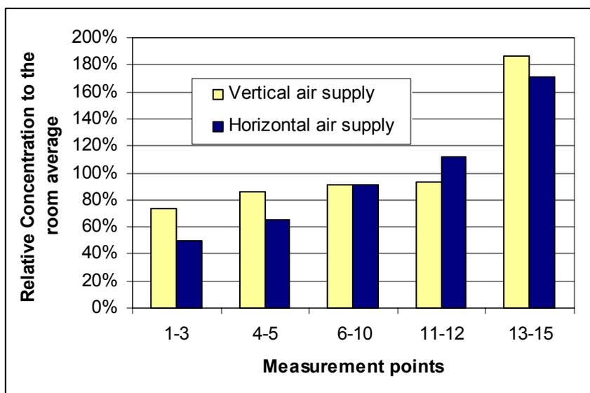
Figure 6. Occupied zone concentration distribution profiles with vertical and horizontal air supply, contaminant source at the east end of the room. Average concentration of measurement points; see location of the points Figure 3.
