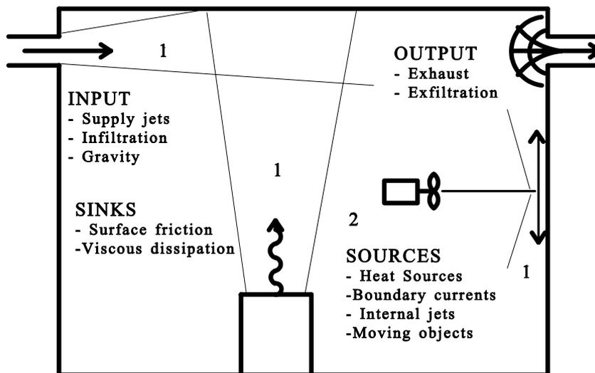
Figure 11. Kinetic energy components and zones in a room space; 1) the jet (supply or thermal) primary zone, 2) the dissipation zone.
