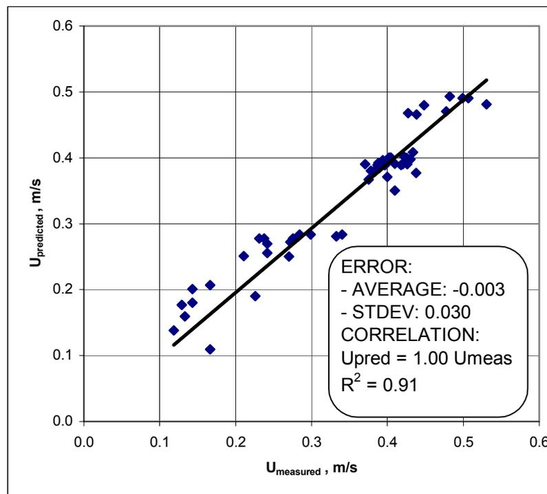
Figure 12. Concentrated supply, Reduced scale, Correlation of measured and predicted occupied zone average velocities, 56 experiments.
