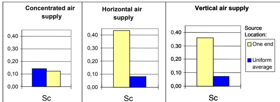
Figure 10. The standard deviation of the contaminant concentrations within the occupied zone with different air diffusion methods. Influence of the contaminant source location non-uniformity.
