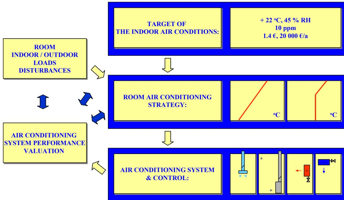
Figure 8. The Room Air conditioning Design and Evaluation Process. Light arrows show the process flow and the dark arrows illustrate the factors to be evaluated during commissioning.
