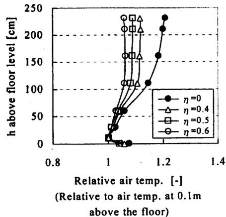
Figure 9. Relative vertical air temperature distribution by  $\eta$  ( $\eta$  = ratio of the cooled ceiling cooling output to the total cooling output) (Tan 1998).
