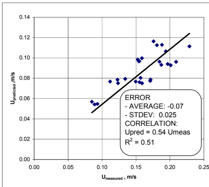
Figure 14. Vertical supply, Correlation of measured and predicted occupied zone average velocities, 27 experiments.
