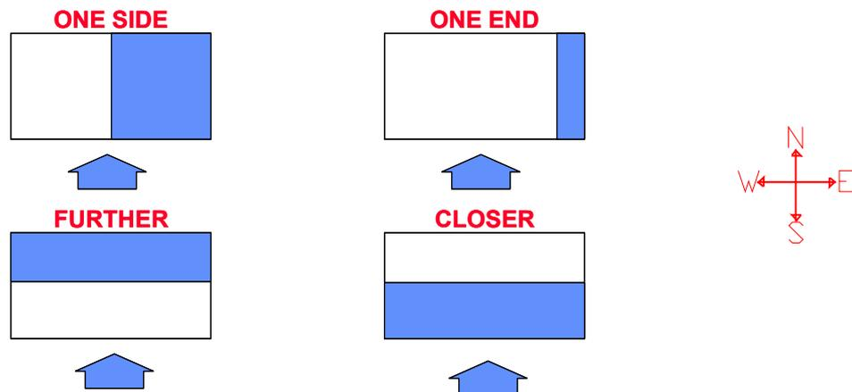
Figure 4. The principle of the room division in source non uniformity studies, horizontal direct supply. The arrows indicate location of the supply air diffusers
