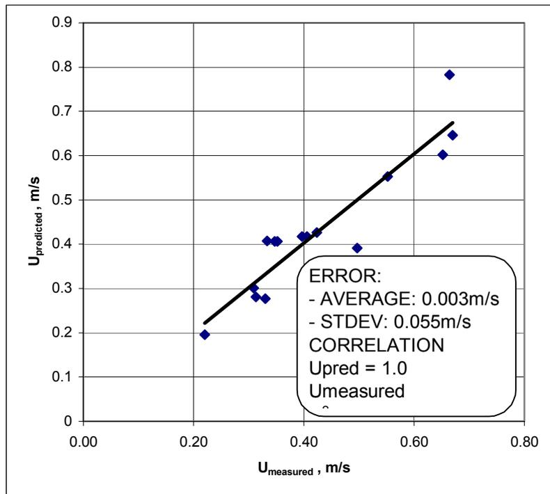
Figure 15. Concentrated jets, full scale, Correlation of measured and predicted occupied zone average velocities, 15 experiments.
