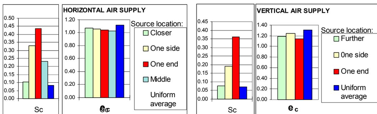
Figure 5. Influence of the contaminant source non uniformity on the occupied zone contaminant concentration standard deviation ( $S_c$ ) and on the contaminant removal effectiveness ( $e_c$ ).
