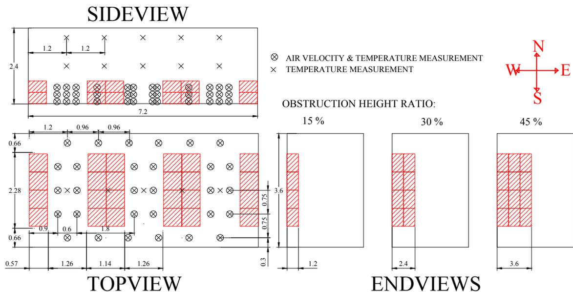
Figure 2. Experimental room layout and air temperature and velocity measurement points, Obstruction area ratio 30%. Dimensions in meters.
