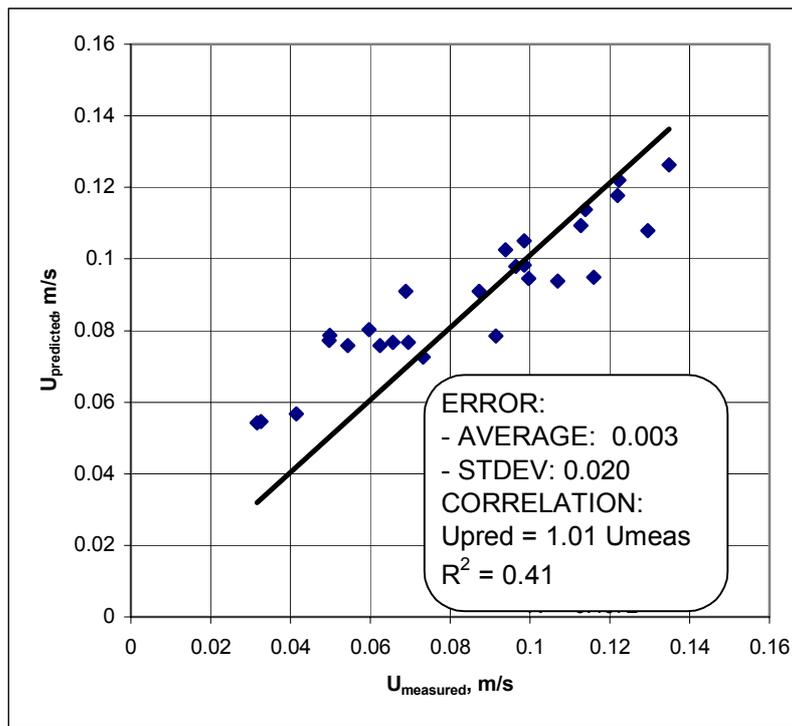
Figure 13. Horizontal direct supply, Correlation of measured and predicted occupied zone average velocities, 30 experiments.
