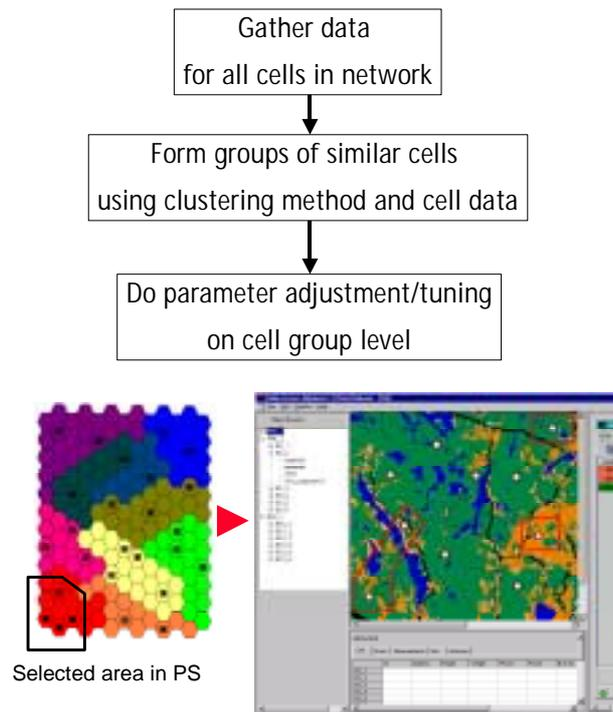
Figure 2. Example of utilisation of cluster information in optimisation process. Selection for cells to be optimised/autotuned. PS stands for performance spectrum.
