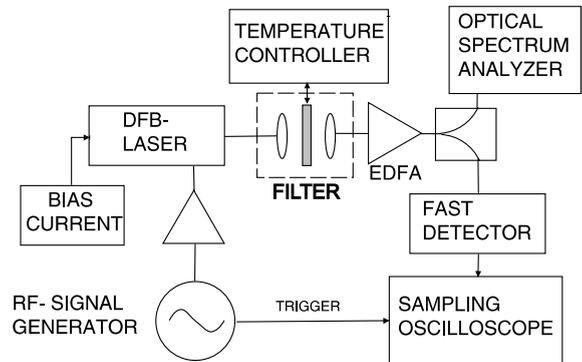
Fig. 1. Experimental setup for generating gain-switched pulses with a DFB laser and for detection of these pulses.
