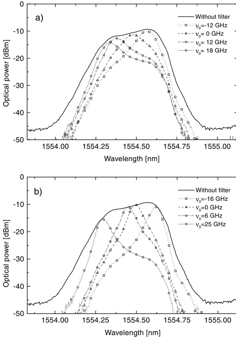
Fig. 2. (a) Measured optical spectra of the gain-switched laser filtered with the filter having a FSR of 110 GHz. (b) Optical spectra of the gain-switched laser filtered with the filter having a FSR of 19 THz. (c) Measured pulse waveforms of the gain-switched laser for several positions of the center frequency of the passband of filter 1. (d) The pulse waveforms of the gain-switched laser filtered with filter 2.
