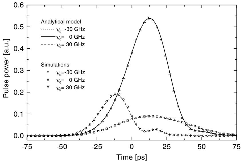
Fig. 3. Calculated intensity of the output pulses for different positions of the filter passband.
