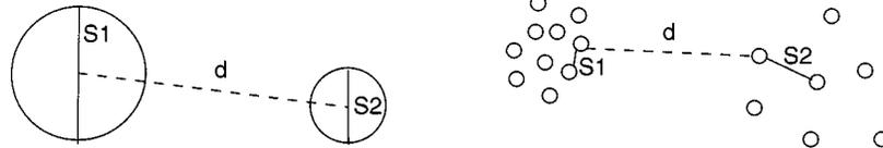
Fig. 3. Different criteria for finding interesting cluster merges: Davies–Bouldin (left) and gap (right). Merge is interesting when  $d > S1 + S2$ , where  $S1$  and  $S2$  are within-cluster distances, and  $d$  is the distance between clusters.
