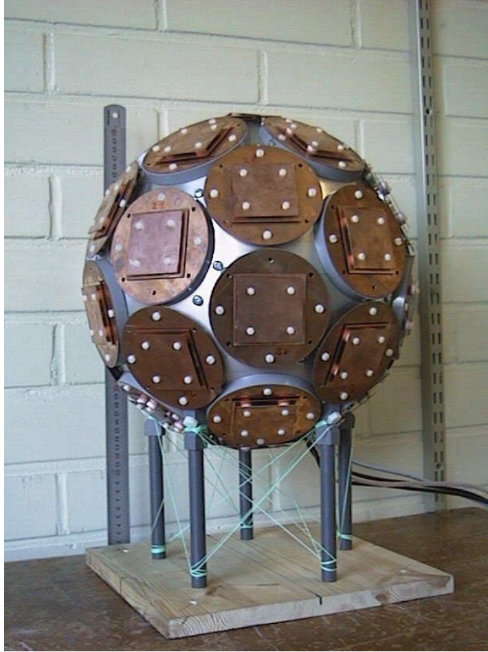
Figure 5. Spherical array for 3-D radio channel measurement at mobile station.
