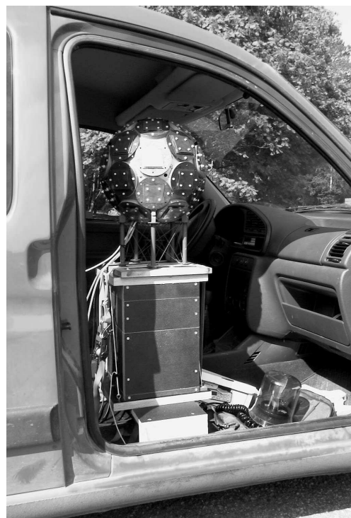
Fig. 2. Spherical array mounting in highway macrocell measurements.
