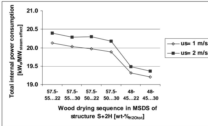
**Figure 18.** Internal power consumption values of integrated drying and boiler-plant systems as functions of drying air velocity through a cross-sectional area of the drying stage (i.e. the slip velocity  $u_s$  in fixed bed operation mode), and of the reduction in wood moisture content. The mass flows of wood dry solids are similar. Process parameters:  $(t_{g,out}-t_s)_i = 8+12$  °C,  $t_{outdoor} = 10$  °C and wood spheres of diameters 20 mm.
