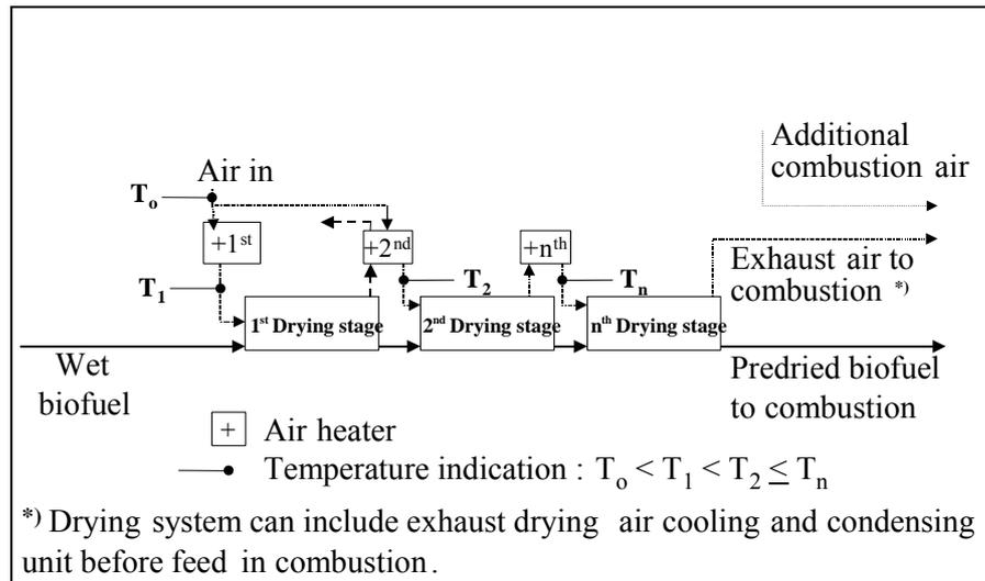
**Figure 4.** The open multistage drying system (MSDS) (Paper II-IV).
