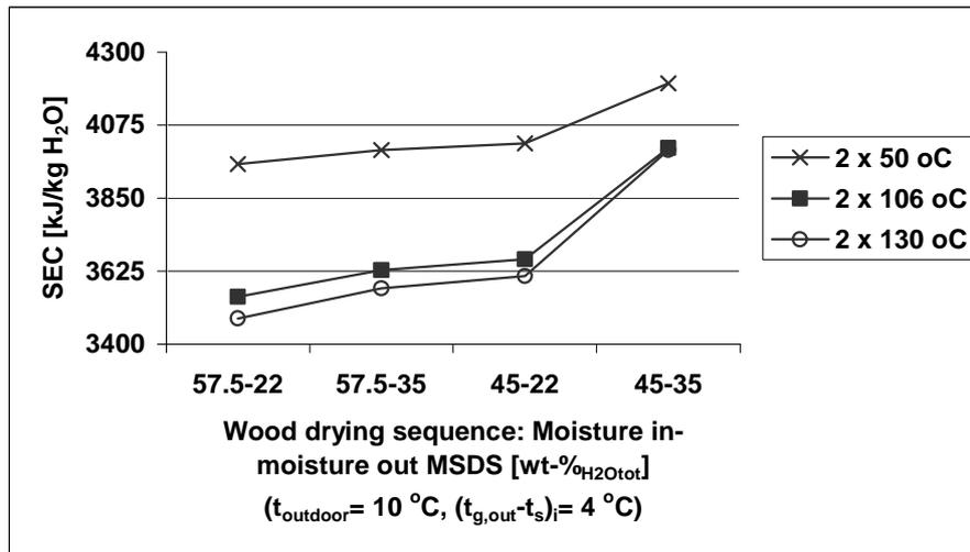
**Figure 11.** Specific energy consumption of MSDSs consisting of two pieces drying stages, as functions of the wood drying sequence (i.e. moisture changes) in MSDSs and of drying air inlet temperature. Equal mass flows of wood dry solids in MSDS.
