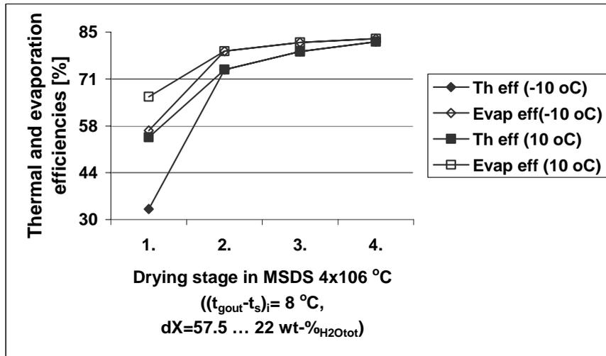
**Figure 14.** Comparison of thermal efficiencies (Th eff) and of evaporation efficiencies (Evap eff) of single drying stages in an MSDS of structure of 4x106 °C drying stages as functions of outdoor air temperature.
