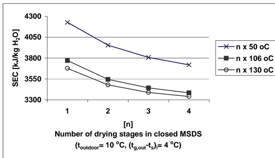
**Figure 9.** Specific energy consumptions (SEC) for the same overall extent of wood drying as a function of the number of drying stages and feed air temperature. Moisture change: 57.5 ... 22 w-%<sub>H<sub>2</sub>O</sub><sub>tot</sub> (1.35 ... 0.28 kgH<sub>2</sub>O/kg DS).
