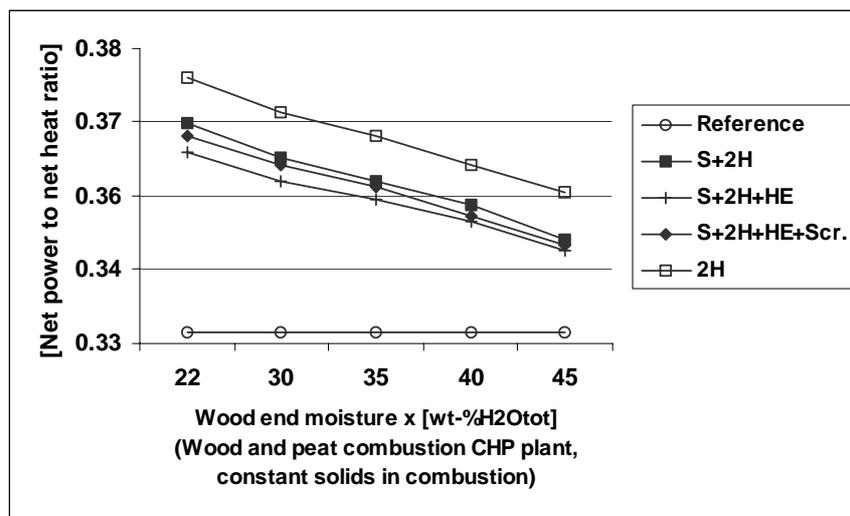
**Figure 16.** Corrected values for the ratios of net output power-to-net output heat of selected CHP plant shown as functions of final wood moisture content and of the structure of the MSDS, which consists of one drying stage heated by secondary energy and two steam heated-drying stages ( Paper IV).
