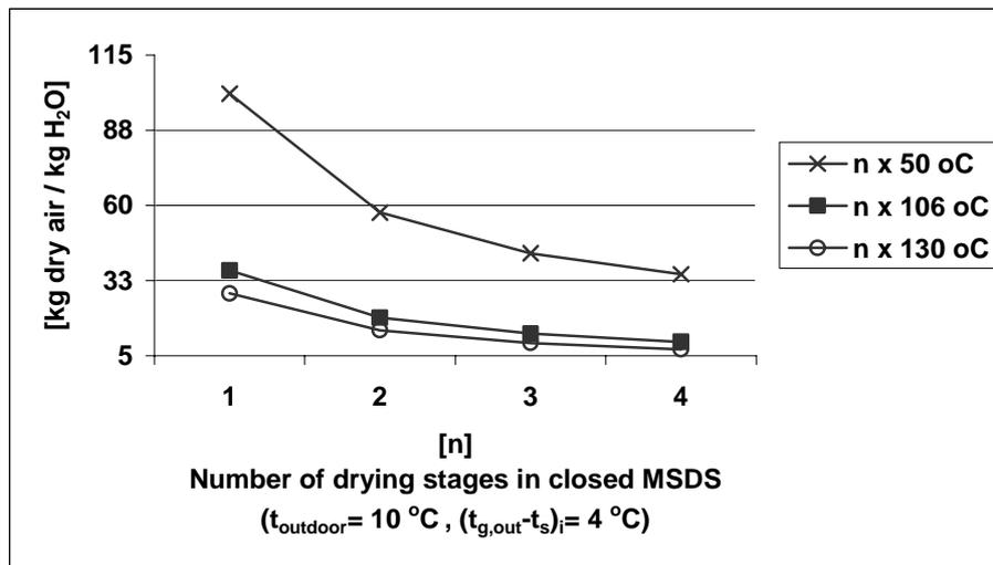
**Figure 8.** Dry air mass flows for the same overall extent of drying as functions of the number of drying stages and feed air temperature. Moisture change: 57.5...22 w-%H<sub>2</sub>O<sub>tot</sub> corresponds to moisture ratios 1.35 ... 0.28 kgH<sub>2</sub>O/kg DS.
