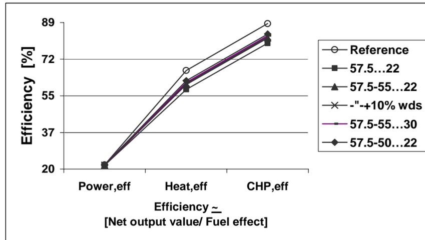
**Figure 15.** CHP efficiencies (for corresponding net values) of different CHP plants as functions of the wood drying sequence in MSDS. One sequence (i.e. 57.5-55...22 wt-% $H_{2O_{tot}}$ ) also includes a ds increase of 10 % as wood in combustion. The fuels in CHP plant boilers are wood and peat [48 wt-% $H_{2O_{tot}}$ ].
