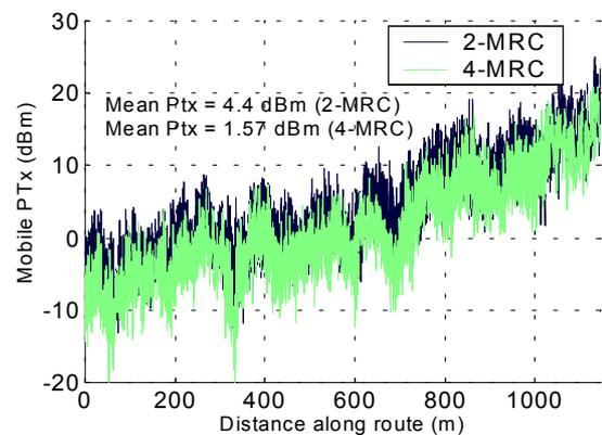
Figure 8. Example of MS Tx power along measurement route.
