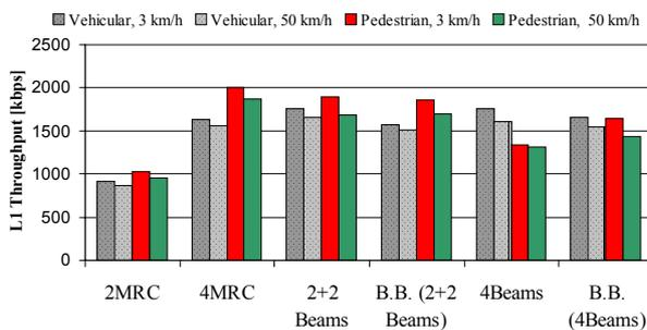
Figure 7. L1 throughput, kbps/carrier/cell.
