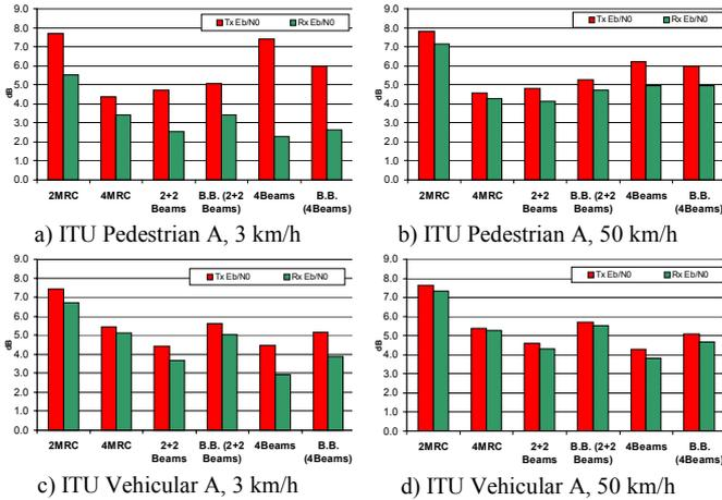
Figure 2. Single link  $E_b/N_0$  performance results with PC for 8 kbps speech service (B.B. between beams,  $C=0.7$ ).
