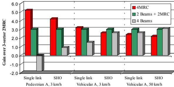
Figure 4. Performance gains in decibels of different antenna configurations compared to corresponding 2MRC values (speech, without PC, FER 1%).
