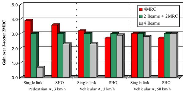
Figure 5. Performance gains in decibels of different antenna configurations compared to the corresponding 2MRC values (packet data, without PC, FER 20%).
