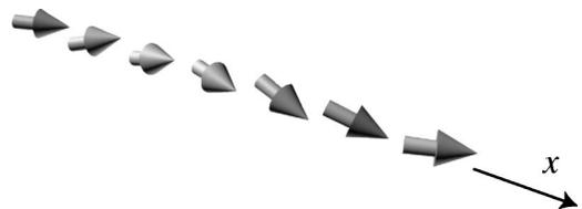
FIG. 2. Variation of  $\hat{\mathbf{I}}$  in a helical texture as a function of  $x$  (Ref. 20). One wavelength  $\lambda$  of the helix is shown.
