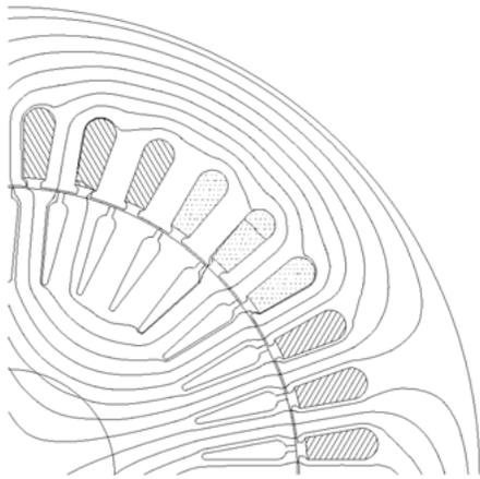
Fig. 2. Cross sectional geometry of the 15 kW motor.
