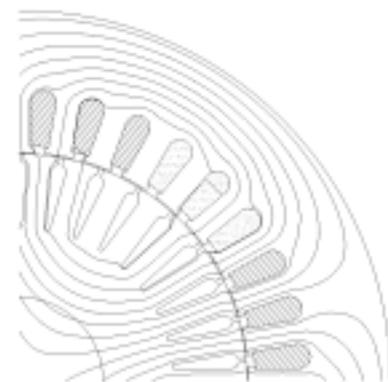
Figure 3. The cross sectional geometry of the 15 kW motor.
