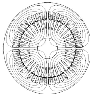
Figure 2. Cross-sectional geometry of the motor studied.
