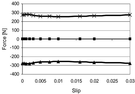
Figure 7. The unbalanced magnetic pull as a function of slip for the motor in the case of 10 % static eccentricity in opposite directions at each end.
