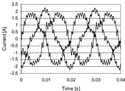
Figure 4. The wave forms of equalising currents of the parallel branches in the stator winding at no-load condition for 10% static parallel eccentricity.
