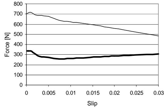
Figure 8. The unbalanced magnetic pull as a function of slip for the motor in the case of 10 % dynamic parallel eccentricity. Thin line is for a series connected and thick line for a parallel connected motor.
