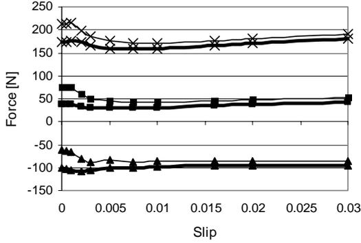
Figure 6. The unbalanced magnetic pull as a function of slip for the motor in the case of 10 % static eccentricity at one end. Thin line is for a series connected and thick line for a parallel connected motor.  $\blacktriangle$  is concentric end  $\blacksquare$  is middle part of the motor and  $\times$  most eccentric end.
