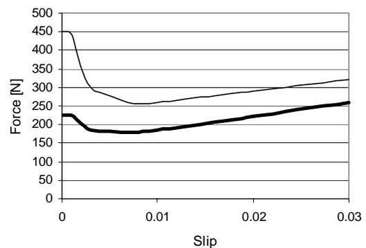
Figure 5. The unbalanced magnetic pull as a function of slip for the induction motor in the case of 10 % static parallel eccentricity. Thin line is for a series connected and thick line for a parallel connected motor.
