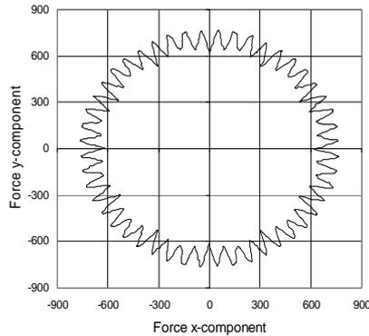
Figure 3. The trace of the magnetic pull vector computed for the 10 % dynamic eccentricity. Rotor is parallel with respect to the stator.
