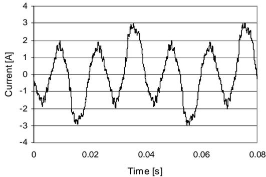
Figure 9. The wave form of an equalising current flowing in the parallel branches of the stator winding at no load condition.
