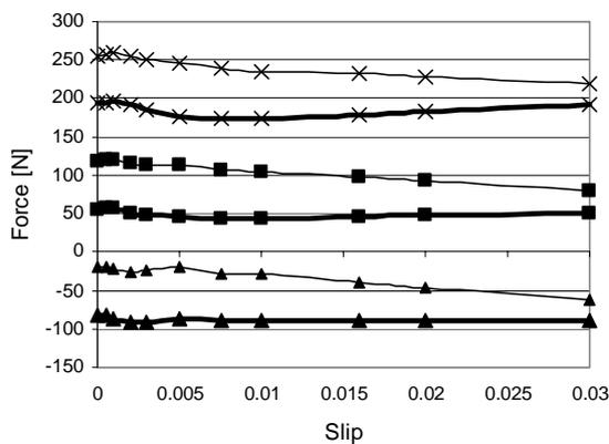
Figure 10. Unbalanced magnetic pull for a one end dynamic eccentricity as a function of slip. Thin line series and thick line parallel connected stator windings.  $\blacktriangle$  is concentric end  $\blacksquare$  is middle part of the motor and  $\times$  most eccentric end.
