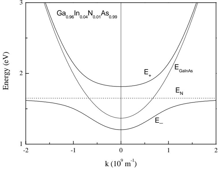
*Figure 3. The conduction band structure of  $\text{Ga}_{0.96}\text{In}_{0.04}\text{N}_{0.01}\text{As}_{0.99}$  near the  $\Gamma$ -point ( $k = 0$ ) calculated with the BAC model. A parabolic approximation for the conduction band of GaInAs was used. The splitting of the conduction band into  $E_-$  and  $E_+$  bands is clearly shown. The energy scale is relative to the top of the valence band.*
