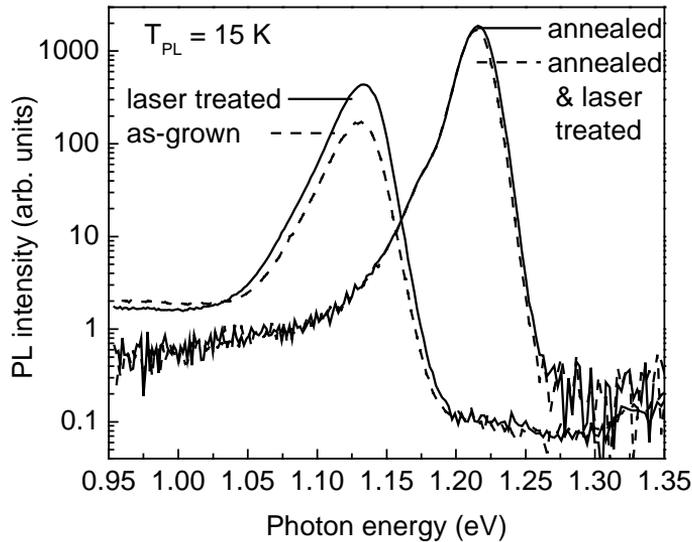
Figure 14. PL spectra measured at 15 K before and after thermal annealing and laser treatment of a  $\text{Ga}_{0.8}\text{In}_{0.2}\text{N}_{0.02}\text{As}_{0.98}$  QW structure. The PL excitation and the laser treatment intensities were  $42 \text{ W/cm}^2$  and  $10000 \text{ W/cm}^2$ , respectively.
