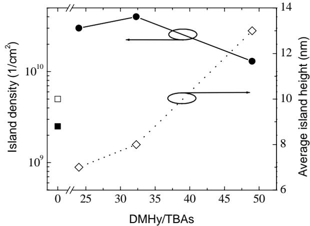
Figure 17. Island density and average island height as a function of DMHy/TBAs ratio for nominally 8-ML-thick  $\text{Ga}_{0.55}\text{In}_{0.45}(\text{N})\text{As}$  QD samples. The squares show the respective data for the reference  $\text{Ga}_{0.55}\text{In}_{0.45}\text{As}$  QD sample.
