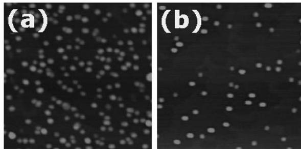
Figure 16. AFM images taken from QD samples grown at 530 °C with (a) 4.5 ML  $\text{Ga}_{0.4}\text{In}_{0.6}(\text{N})\text{As}$  and (b) 4.5 ML  $\text{Ga}_{0.4}\text{In}_{0.6}\text{As}$ . The scan size is  $0.5 \times 0.5 \mu\text{m}^2$ .
