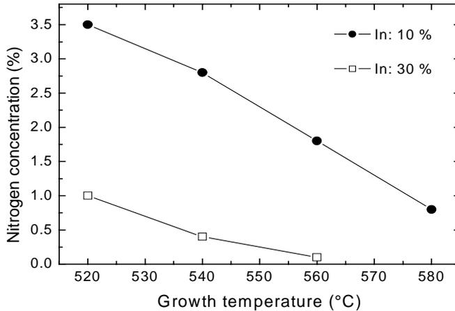
Figure 9. Effect of growth temperature on the N concentration for In concentrations of 10 and 30 % in GaInNAs MQW structures.
