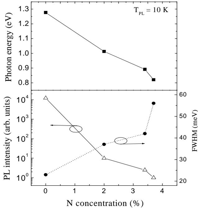
Figure 11. Low-temperature PL data from  $Ga_{0.778}In_{0.228}N_xAs_{1-x}$  MQW structures as a function of the N concentration. The PL peak energy and the PL intensity decrease and the FWHM increases with increasing N concentration.
