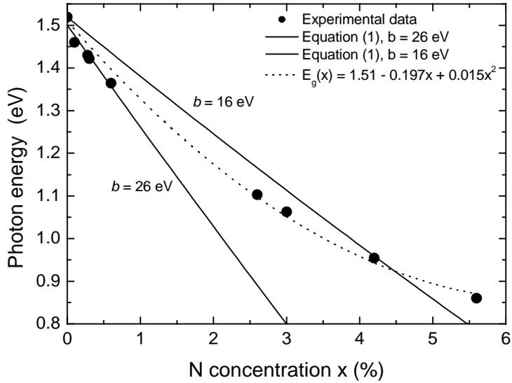
Figure 2. Photoluminescence peak energies for  $\text{GaAs}_{1-x}\text{N}_x$  ( $0 \leq x \leq 5.6$  %) samples measured at the temperature of 9 K. The solid lines are the bandgap energies fitted to data with a bowing parameter  $b$  of 16 and 26 eV for the average and the low N composition, respectively. For comparison, the dotted line shows a fit with a quadratic function.
