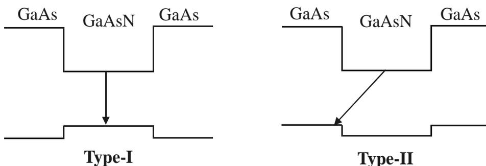
*Figure 4. Schematic representation of band alignment in type-I and type-II quantum structures. The arrows show dominant recombination transitions, *i.e.*, direct in space for type-I transitions and indirect in space for type-II transitions. Both band alignments have been proposed for GaAsN/GaAs quantum structures, but recent results strongly favor the type-I band alignment.*
