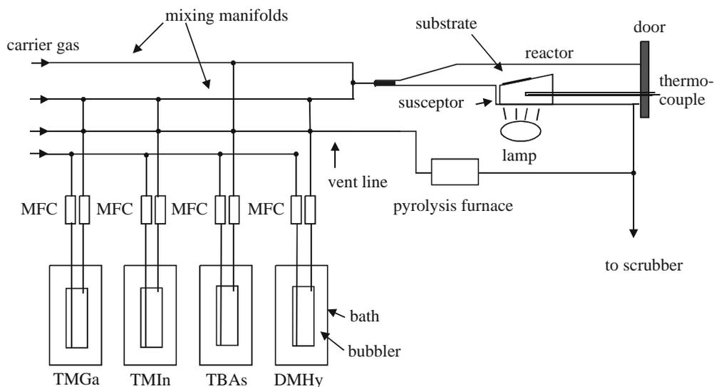
Figure 5. Schematic representation of the MOVPE apparatus.
