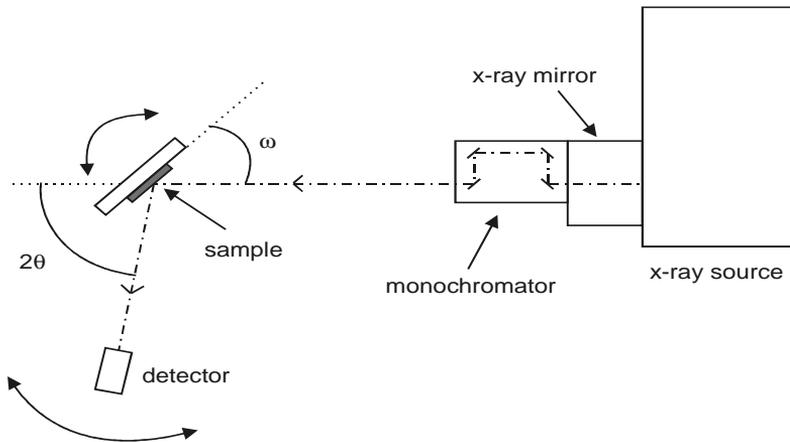
Figure 8. Schematic representation of the x-ray diffraction measurement setup. The angle between the incident beam and the sample surface is  $\omega$  and the angle between the incident beam and the diffracted beam is  $2\theta$ .
