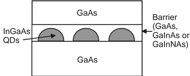
*Figure 18. Schematic illustration of the  $\text{Ga}_{0.5}\text{In}_{0.5}\text{As}$  QDs grown on GaAs and embedded in a  $\text{Ga}_{1-y}\text{In}_y\text{N}_x\text{As}_{1-x}$  barrier layer with different compositions. The  $\text{In}$  and  $\text{N}$  concentrations were varied in the range of  $0 \leq y \leq 0.25$  and  $0 \leq x \leq 0.035$ , respectively. The thickness of the barrier layer was either 5 or 10 nm.*
