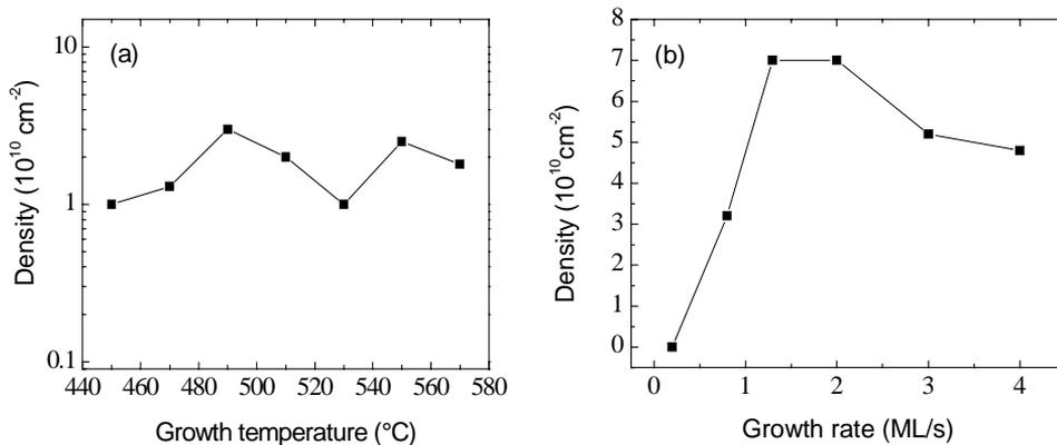
Figure 15. Island density of Ga<sub>0.4</sub>In<sub>0.6</sub>(N)As samples as a function of (a) growth temperature and (b) growth rate.
