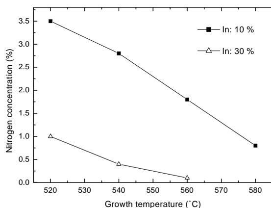
Fig. 2. Effect of growth temperature on the N concentration for two In concentrations of 10% and 30%. The N concentration increases when the growth temperature is decreased and the maximum is achieved at 520°C. Increase in the In concentration results in decrease of the N concentration.
