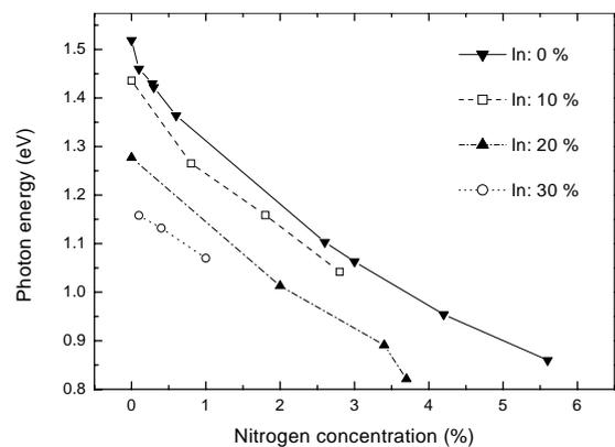
Fig. 1. LTPL peak energies of the  $\text{Ga}_{1-x}\text{In}_x\text{N}_y\text{As}_{1-y}$ (10 nm)/GaAs(30 nm) MQW samples fabricated with different In concentrations. A slight reduction in the band gap bowing is observed for N concentrations of less than 1% when the In concentration is increased.
