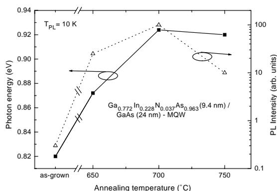
Fig. 6. PL peak energies and intensities of a MQW structure after post-growth annealing at different temperatures for 10 min. The PL peaks blueshift for all annealing temperatures. Annealing at 700 °C increases the PL intensity over two orders of magnitude.
