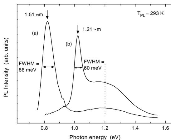
Fig. 8. RTPL spectra of two annealed MQW structures. (a)  $\text{Ga}_{0.74}\text{In}_{0.26}\text{N}_{0.03}\text{As}_{0.97}(9\text{ nm})/\text{GaAs}(24.5\text{ nm})$  and (b)  $\text{Ga}_{0.772}\text{In}_{0.228}\text{N}_{0.02}\text{As}_{0.98}(9.5\text{ nm})/\text{GaAs}(26.5\text{ nm})$ . The PL spectrum of the sample (a) peaks at 0.82 eV (1.51  $\mu\text{m}$ ).
