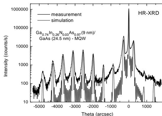
Fig. 3. Measured and simulated X-ray rocking curves of a  $\text{Ga}_{0.74}\text{In}_{0.26}\text{N}_{0.03}\text{As}_{0.97}(9\text{ nm})/\text{GaAs}(24.5\text{ nm})$  MQW structure.
