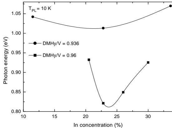
Fig. 4. Dependence of the PL peak energy on the In concentration with two different DMHy/V ratios. There exists an optimum window at the In concentration of around 23% for the smallest PL peak energies.
