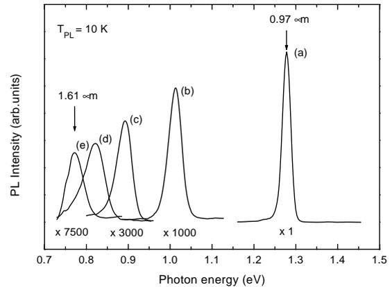
Fig. 5. LTPL spectra of  $\text{Ga}_{1-x}\text{In}_x\text{N}_y\text{As}_{1-y}$ (9 nm)/GaAs(24.5 nm) MQW samples fabricated with different DMHy/V ratios. The In and N concentrations of the samples are: (a)  $x = 0.228$  and  $y = 0$ , (b)  $x = 0.228$  and  $y = 0.02$ , (c)  $x = 0.228$  and  $y = 0.034$ , (d)  $x = 0.228$  and  $y = 0.037$  and (e)  $x = 0.26$  and  $y = 0.03$ . The PL spectrum of the sample (e) peaks at 0.77 eV (1.61  $\mu\text{m}$ ).
