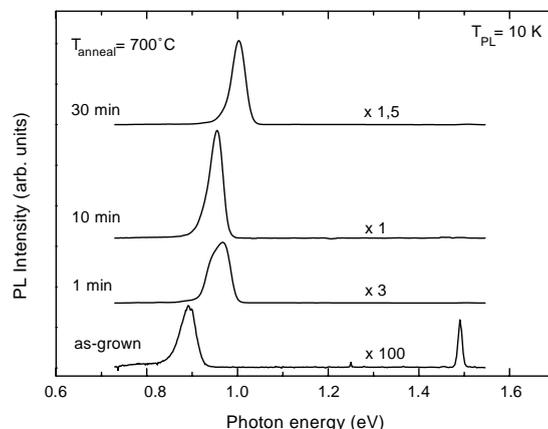
Fig. 7. PL spectra of a  $\text{Ga}_{0.772}\text{In}_{0.228}\text{N}_{0.034}\text{As}_{0.966}(10\text{ nm})/\text{GaAs}(24.3\text{ nm})$  MQW structure annealed at 700 °C for different times. Annealing for longer times than 10 min does not enhance the PL intensity further, but results in larger blue shift of the PL peak.
