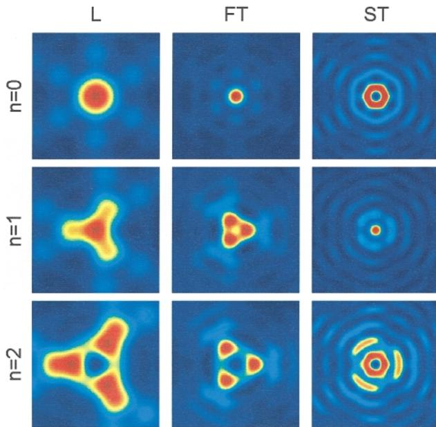
FIG. 1 (color). Nondiffracting acoustic beams in quartz. The left column shows the L mode for  $n = 0, 1,$  and  $2,$  the middle one illustrates the FT mode, and the right column is the ST mode. Color shading denotes the time-averaged kinetic energy; each frame represents  $100 \mu\text{m} \times 100 \mu\text{m}$  area.
