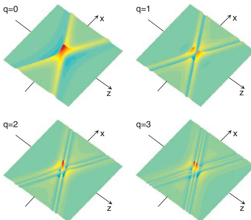
**Figure 2.** First four orthogonal X waves,  $\Phi_{n,q}^{\text{ort}}$ . Orthogonal X waves feature an increasing number of ‘halo wave fronts’ (or ‘halo toroids’ [8]), required for making the scalar product between different wave modes vanish.
