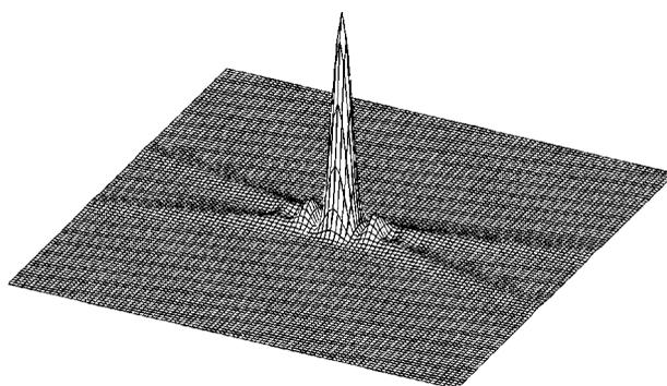
**Figure 4.** Intensity of the Bessel-X pulse as given by equation (21) with 20 terms to be compared with figure 1(a) in [5]. The pulse duration (FWHM) is 3 fs, carrier frequency  $\omega_0 = 3.14 \times 10^{15} s^{-1}$  and  $\alpha = 6.2$  fs. The area illustrated in this meridional plane is  $20 \times 20 \mu m^2$ .
