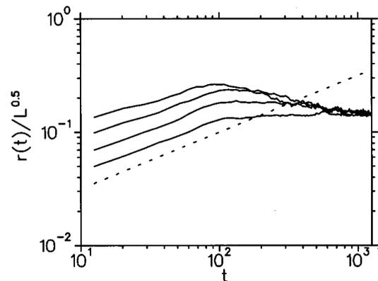
FIG. 12. Averaged wave-front roughness as a function of time in TLM lattices with  $p=0.85$  and vertical heights  $L_y=30,60,120,240$ ; the driving frequency is 0.314. The dashed line is given by  $r(t) \propto t^{1/2}$ .
