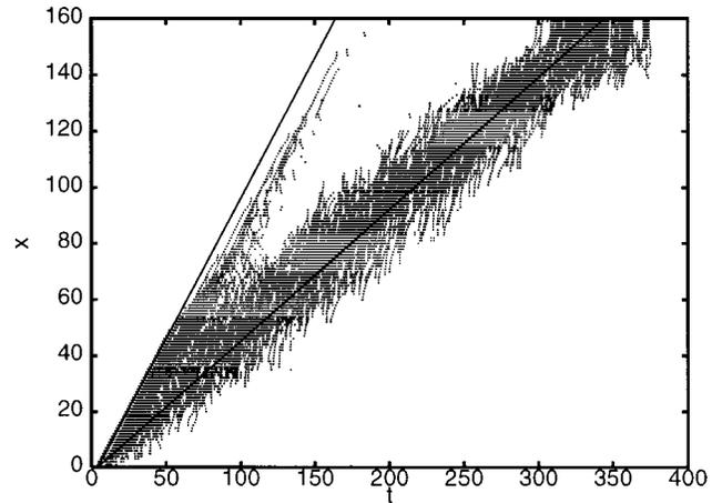
FIG. 6. Distance of the sites in a network of size  $160 \times 160$  as a function of the time when the site reaches its first displacement maximum with  $l=1$ ,  $m=0.01$ ,  $w=0.1$ ,  $E=1.0$ ,  $p=0.9$ , and the frequency 0.0125. The lines are given by Eq. (3) with  $p=0.9$  and  $p=1$ .
