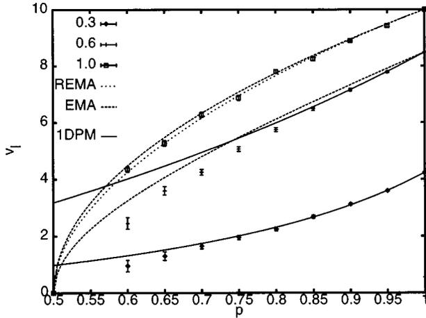
FIG. 1. Average wave-front propagation velocities of longitudinal waves in lattices with  $l=1$ ;  $m=0.005, 0.01$ ;  $w=0.3, 0.6, 1.0$ ;  $E=1.0$ ; and the frequency 0.125. The corresponding velocities calculated from the effective-medium approximation (EMA) and the one-dimensional path model (1DPM) are shown by dotted and solid lines, respectively.
