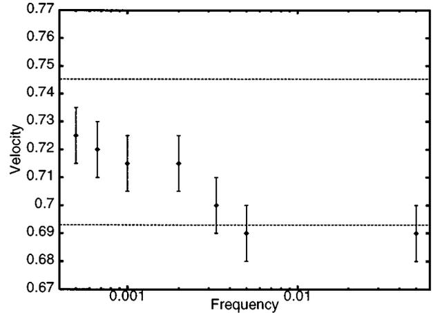
FIG. 3. Average velocity of a longitudinal wave front as a function of the driving frequency with  $l=1$ ,  $m=0.1$ ,  $w=0.3$ ,  $p=0.9$ , and  $E=1.0$ . The upper and the lower lines are the prediction by the effective-medium approximation and the model of one-dimensional paths, respectively.
