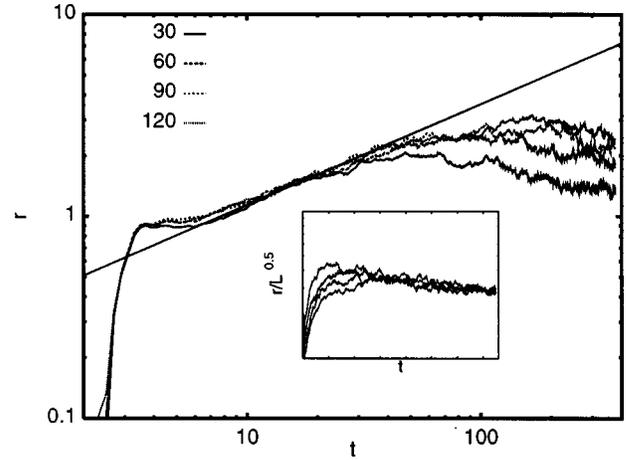
FIG. 11. Averaged wave-front roughness as a function of time in lattices with  $p=0.7$  and vertical heights  $L_y=30,60,90,120$ ;  $l=1$ ,  $m=1.0$ ,  $w=1.0$ ,  $E=1.0$ , and the frequency is 0.125. The fitted line is given by  $r(t) \propto t^{1/2}$ . The inset shows the same data on a semilogarithmic scale, with the y axis rescaled by  $L^{-0.5}$ .
