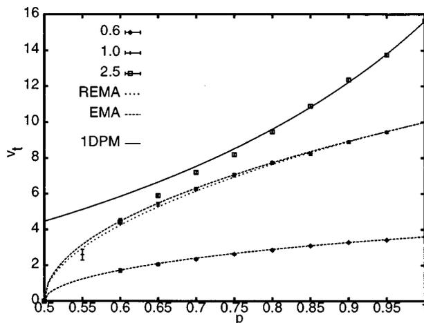
FIG. 2. Average wave-front velocities of transverse waves in lattices with  $l=1$ ;  $m=0.01, 0.06$ ;  $w=0.6, 1.0, 2.5$ ;  $E=1.0$ ; and the frequency 0.0125. The corresponding velocities calculated from the EMA and the 1DPM are shown by dotted and solid lines, respectively.
