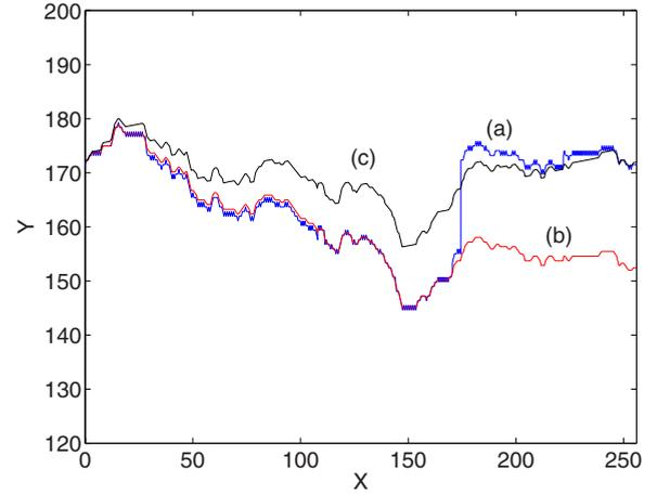
FIG. 3. (Color online) Figure shows a typical single valued crack profile  $h(x)$  with jumps based on solid-on-solid projection scheme [identified as (a)]. Removing the jumps in the crack profile  $h(x)$  makes it a nonperiodic profile [identified as (b)]. Subtracting a linear profile from this nonperiodic profile results in a periodic profile [identified as (c)].
