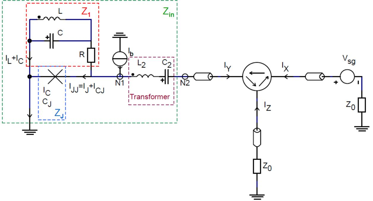
FIG. 1. Amplifier circuit with a Josephson junction denoted by the cross. Node N1 specifies the node to which the bias current  $I_b$  is fed. A circulator connects the branches X, Y, and Z in a manner denoted by the arrows; the amplifier input impedance  $Z_{in}$  is the impedance at N2 looking outward from port Y. The junction has internal capacitance  $C_J$  which is not drawn explicitly. For the variables, see text.
