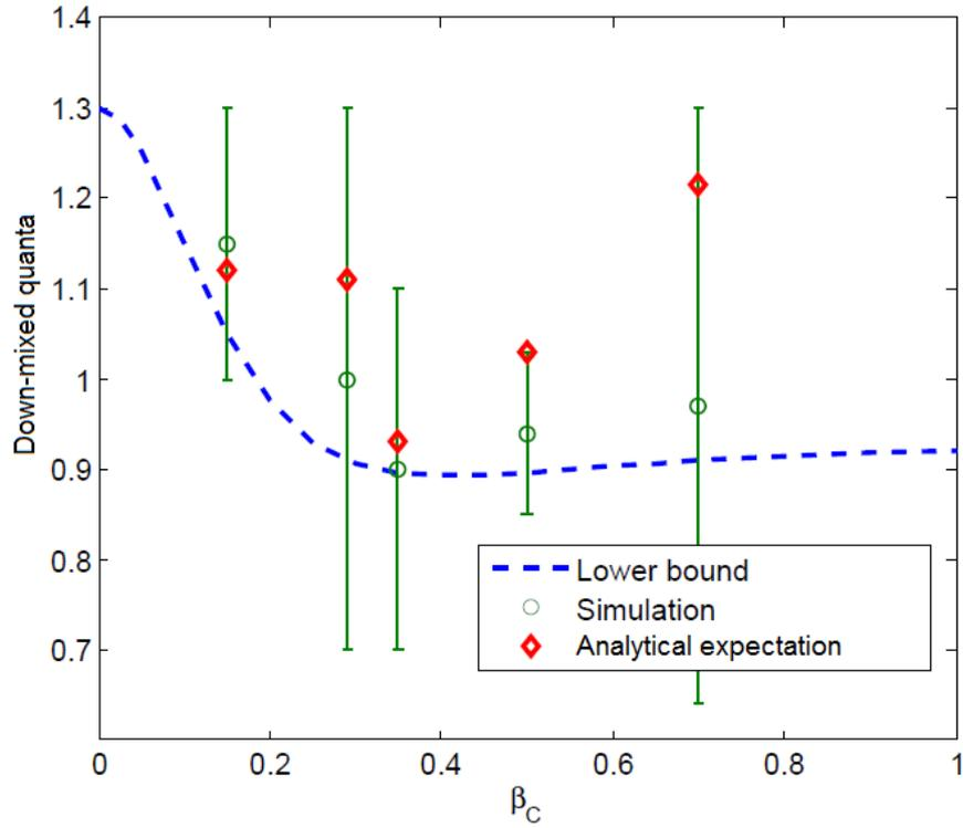
FIG. 4. Analytic model, Eqs. (61) and (62), yields a lower bound for added noise as a function of  $\beta_C$ . Several SJAs with varying parameters were simulated at  $v_b = 3$ . Gain was in the range  $G_m = 11.2 - 24.5$  dB and  $N = \omega_J/\omega_s = 2.3 - 5.6$ . Our analytic model predicts accurately the down-mixed noise contribution provided that  $\omega_J > \omega_p$  and  $RC_J$  is small.
