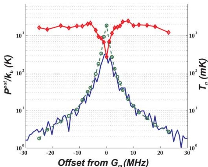
**Figure 4** | The effective output noise temperature  $P_n^{\text{out}}/k_B$  (left scale) is compressed in the simulation (denoted by solid blue line) when compared with the product of the simulated gain ( $G - 1$ ) and the uncompressed down-mixed noise of  $2.4 \text{ K} \times k_B$  from Eq. 3 (○). After dividing the simulated output spectrum by the calculated gain, a clear dip is revealed in the input noise temperature (◇, right scale).
