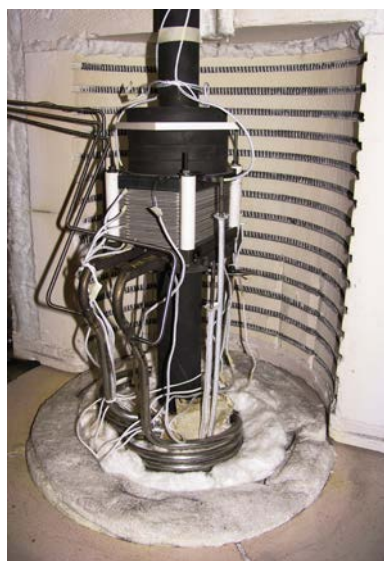
Fig. 2. The 30-cell stack before testing.
