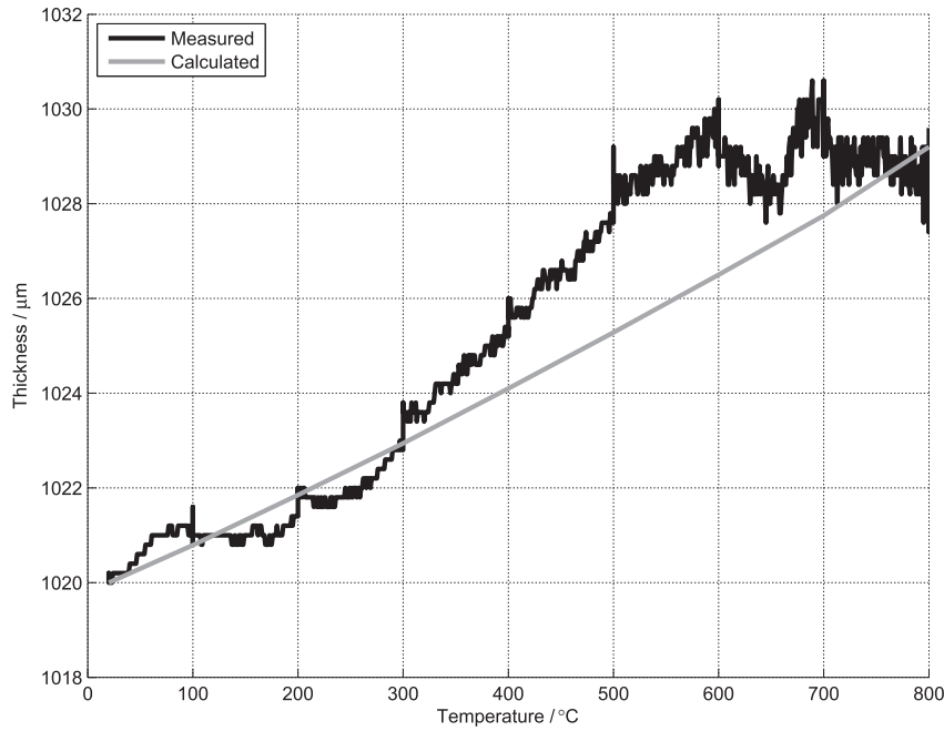
Fig. 2. Measured thickness of Crofer 22H plate (1020 μm initial thickness) as a function of temperature together with calculated thickness based on manufacturers datasheet.
