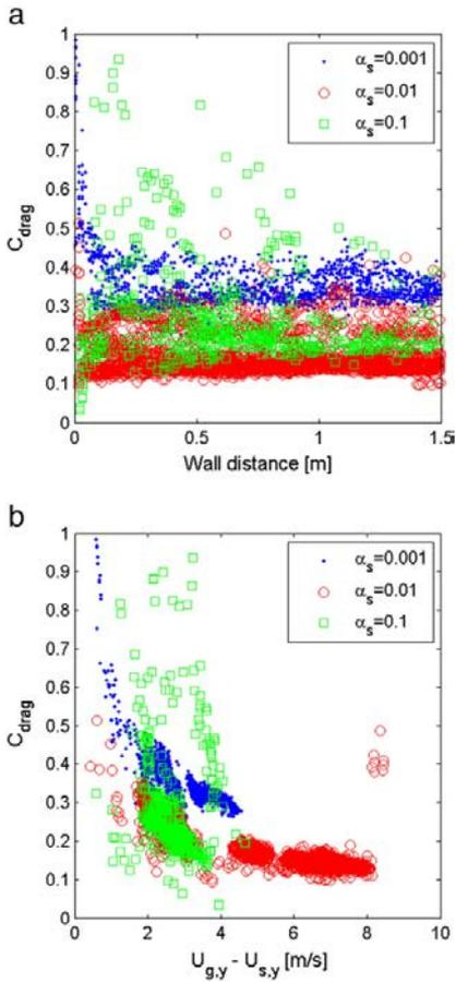
Fig. 9. Summarized data for Cases 9, 10, 11, 12, 13, 14 and 17 at solid volume fractions 0.001, 0.01 and 0.1. a) Drag correction coefficient  $C_{drag}$  plotted as a function of the distance to the wall,  $\Delta x_{wall}$ . b) Drag correction coefficient  $C_{drag}$  plotted as a function of the slip velocity.
