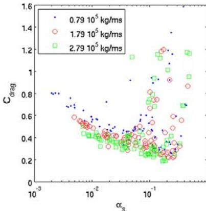
Fig. 14. Effect of gas viscosity on  $C_{drag}$  (Cases 8, 3, and 7, respectively, in Table 1).
