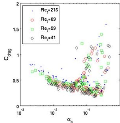
Fig. 11. Effect of Reynolds number (calculated on the basis of particle terminal velocity) on  $C_{drag}$  (Cases 8, 5, 6, and 7, respectively, in Table 1). Archimedes numbers for the four cases are 27200, 6900, 3720, and 2180, respectively.
