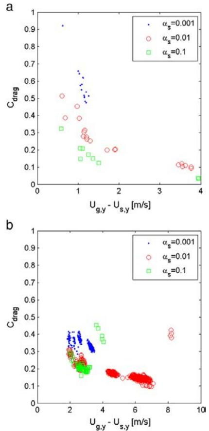
Fig. 10. Summarized data from Cases 9, 10, 11, 12, 13, 14 and 17. Drag correction coefficient  $C_{drag}$  plotted as a function of the slip velocity at three different solid volume fractions a) in the wall layer and b) in the central region.
