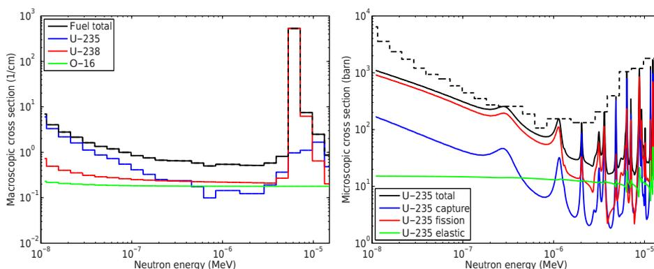
**Figure 1. Left(a): Macroscopic multi-group cross sections used for sampling the target nuclide after collision in fuel. Right(b): Microscopic cross sections used for rejection sampling and selecting the reaction mode. The number of energy groups has been significantly reduced in this example for the sake of clarity.**
