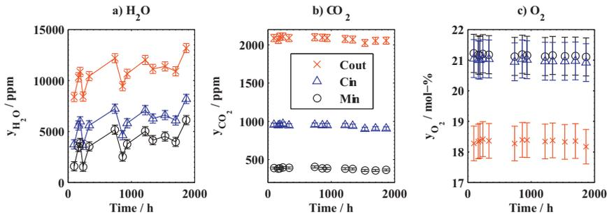
Fig. 3 Measured fraction of a) H<sub>2</sub>O, b) CO<sub>2</sub>, and c) O<sub>2</sub> in the cathode gas at (○) module inlet *Min*, (△) cathode inlet *Cin* and (×) cathode outlet *Cout*. System at nominal operating conditions with stack current at 200 A.
