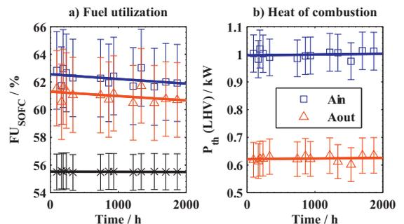
Fig. 8 a) SOFC stack fuel utilisation, and b) heat of combustion due to diffusive anodic leakages with ( $\square$ )  $A_{in}$  and ( $\triangle$ )  $A_{out}$  gas composition. ( $\times$ ) Ideal fuel utilisation without leakages. A linear fit is shown as a solid trend line.
