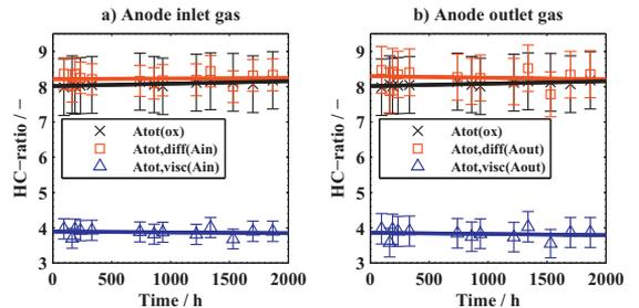
Fig. 6 HC-ratio of the anodic leakage determined by (x) air system measurements, (□) diffusive leakage model, and (Δ) viscous leakage model, with a)  $Ain$  and b)  $Aout$  gas composition. A linear fit is shown as a solid trend line.
