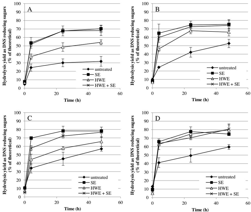
**Fig. 2.** Hydrolysis of pretreated spruce bark in 1% consistency in 50 mM acetate buffer, pH 5 at 45 °C. Pretreatments used were hot water extraction (HWE), steam explosion (SE) and combination of the two (HWE + SE). Hydrolysis with: (A) Low dosage of cellulase and  $\beta$ -glucosidase, (B) low dosage of cellulase and  $\beta$ -glucosidase, high dosage of pectinase, (C) high dosage of cellulase and  $\beta$ -glucosidase, (D) high dosage of cellulase,  $\beta$ -glucosidase and pectinase.
