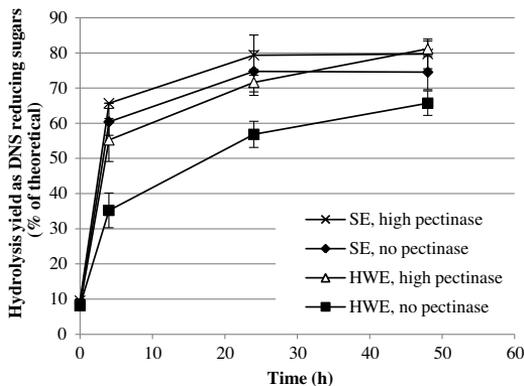
**Fig. 3.** Hydrolysis of pretreated spruce bark with low cellulase dosage, high  $\beta$ -glucosidase dosage and with or without pectinase in 1% consistency in 50 mM acetate buffer, pH 5 at 45 °C. Pretreatments used were hot water extraction (HWE) and steam explosion (SE).
