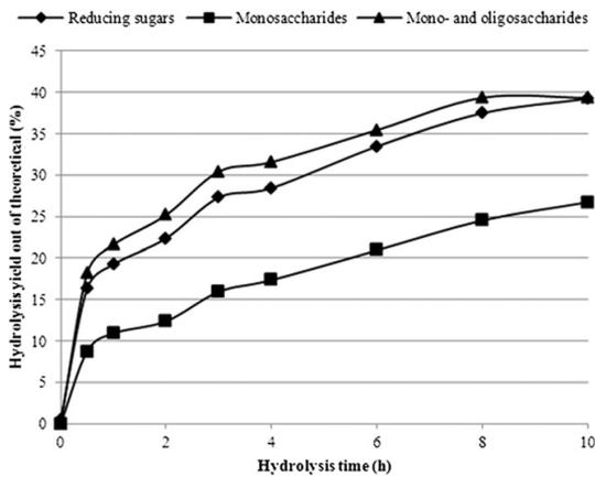
**Fig. 4 – Hydrolysis yield as reducing sugars, monosaccharides (HPLC analysis), and mono- and oligosaccharides (HPLC analysis after secondary acid hydrolysis of the supernatant) in liquefaction of waste fibre with 8 FPU g<sup>-1</sup> in 300 g kg<sup>-1</sup> substrate concentration, 50 °C and pH 5.**
