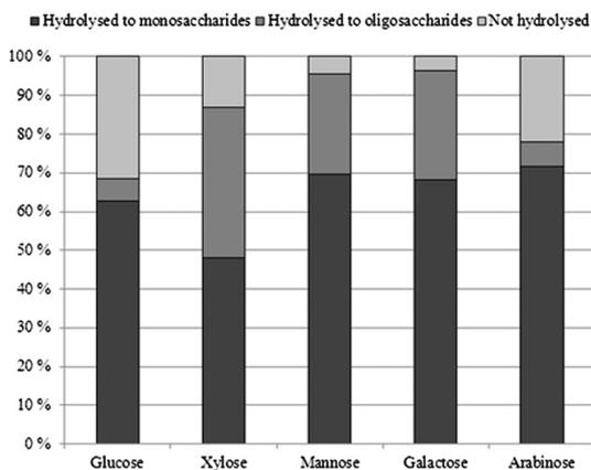
**Fig. 5 – Hydrolysis yield of monosaccharides after 10 h liquefaction of waste fibre with 8 FPU g<sup>-1</sup> in 300 g kg<sup>-1</sup> substrate concentration, 50 °C and pH 5.**
