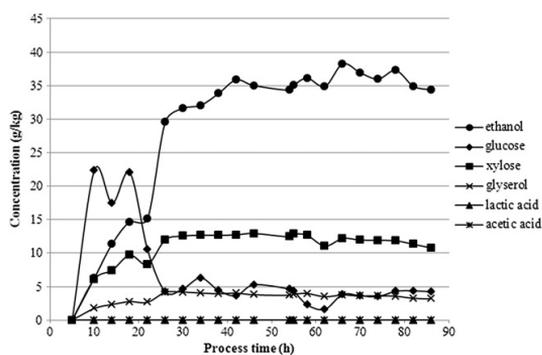
**Fig. 6 – The main substrate and metabolite concentrations during a continuous SSF process with waste fibre after continuous 6 h liquefaction in 300 g kg<sup>-1</sup> substrate concentration.**
