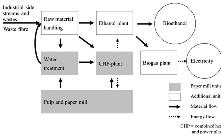
**Fig. 1** – The FibreEtOH concept consists of raw material handling including the fractionation of SRF, liquefaction and fermentation of the feedstocks, distillation and absorption of ethanol, biogas and electricity production from the fermented residue, and a shared water treatment and a combined heat and power (CHP) plant with a pulp and paper mill.
