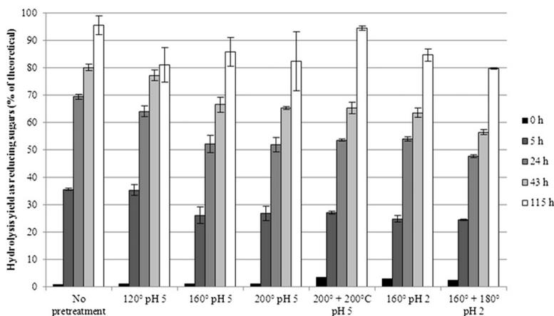
**Fig. 3 – The effect of thermal and acidic pre-treatment to hydrolysis yield of waste fibre with  $10 \text{ FPU g}^{-1}$  cellulase and  $1000 \text{ nkat g}^{-1}$   $\beta$ -glucosidase in  $100 \text{ g kg}^{-1}$  substrate concentration,  $100 \text{ mol m}^{-3}$  sodium acetate buffer pH 5 at  $45^\circ\text{C}$ . Error bars show the standard deviation of triplicate samples.**
