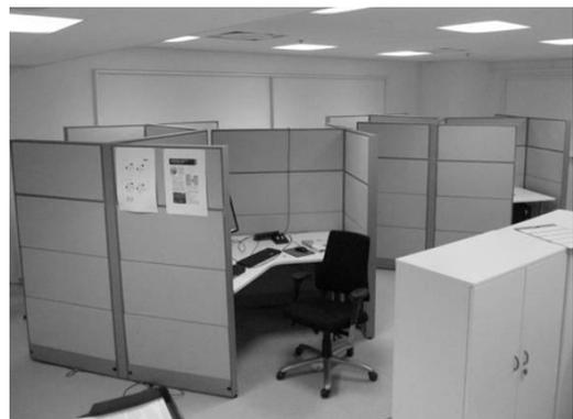
Figure 2. View of the office laboratory when the screen height was 1.7 m. Two other screen heights were also investigated. The wall absorbers were not installed.
