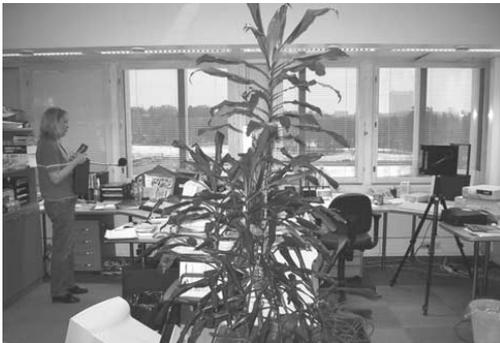
Figure 6. Measurement of *RASTI* between two workstations. The screen is situated behind the palm tree. The source apparatus is on the right side.
