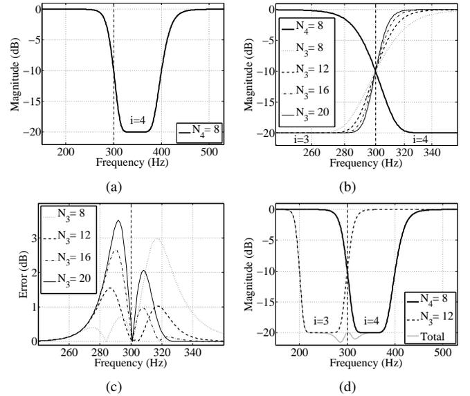
Fig. 3. Example of the interaction around the transition band of two adjacent band filters: (a) the magnitude response of the band 4 filter, (b) the same band 4 filter as well as four candidate filters for the adjacent band with different orders, (c) the absolute error around the transition band between bands 3 and 4, and (d) the magnitude response of the best matching filter along with the original band 4 filter and their combined response (gray curve).
