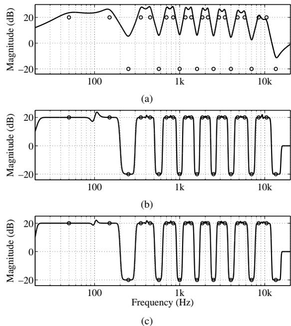
Fig. 5. Magnitude response of (a) a second-order Regalia-Mitra ( $N = 48$ ), (b) a non-optimized ( $N = 384$ ), and (c) an optimized graphic equalizer ( $N = 328$ ). The circles indicate the command points of the graphic equalizer.
