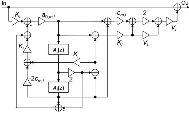
Fig. 2. The  $m^{\text{th}}$  fourth-order section of the  $i^{\text{th}}$  band filter [4], [15].
