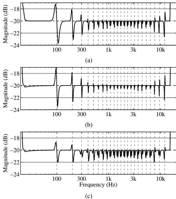
Fig. 4. Comparison of the magnitude responses of different Bark-band graphic equalizer filter orders, where (a) and (b) are the responses of non-optimized graphic equalizers with orders  $N = 384$  and  $N = 672$ , respectively, and (c) is the response of the equalizer optimized with the proposed algorithm ( $N = 328$ ). The solid horizontal lines indicate the  $\pm 2$  dB tolerances. The target gain is  $-20$  dB in the frequency range of interest.
