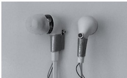
**Fig. 2:** Headset prototype with microphones attached outside each earpiece.
