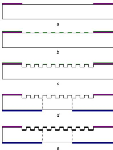
**Figure 2** Process flow for the fabrication of square profile flowfield body with gas inlets, flowfield and gas diffusion layer
