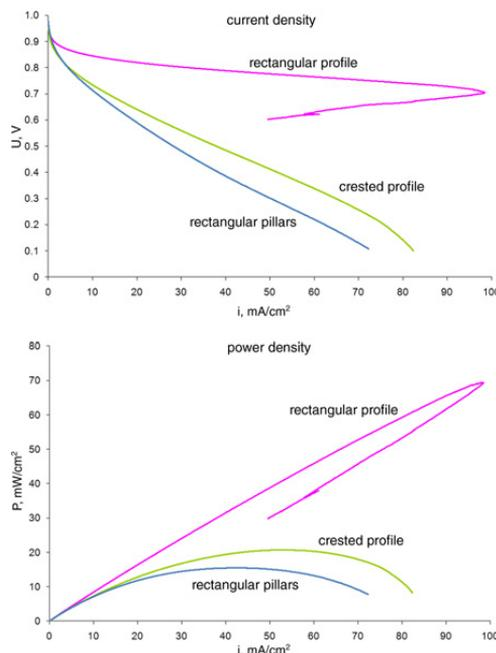
**Figure 6** Measured current and power density plots for all three types of micro fuel cells
