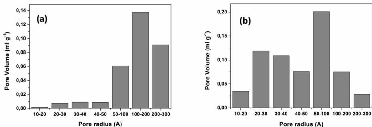
**Fig. 5. Pore size distribution of PtRu-Vulcan (a) and PtRu-FWCNTs (b).**
