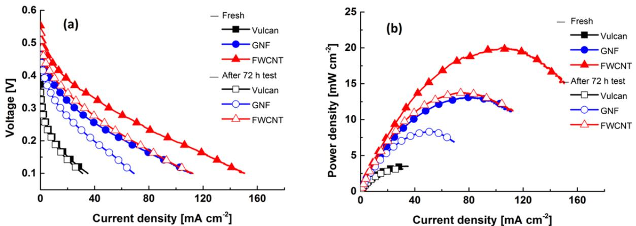
**Fig. 6. Polarization curves of current density (a) and power density (b) of PtRu-Vulcan, PtRu-GNFs and PtRu-FWCNTs anodes, before and after the 72 h CA measurements.**
