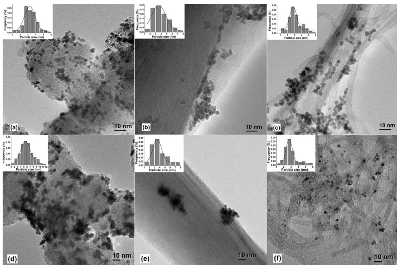
**Fig. 10.** HR-TEM images and the corresponding PtRu particle size distribution histograms on the fresh supports: Vulcan (a), GNFs (b) and FWCNTs (c), and on the used ones: Vulcan (d), GNFs (e) and FWCNTs (f).
