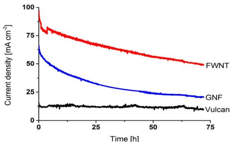
**Fig. 7. CA measurements in Si-MFCs with PtRu anode catalysts supported on Vulcan, GNFs and FWCNTs for 72 h at 0.2V.**
