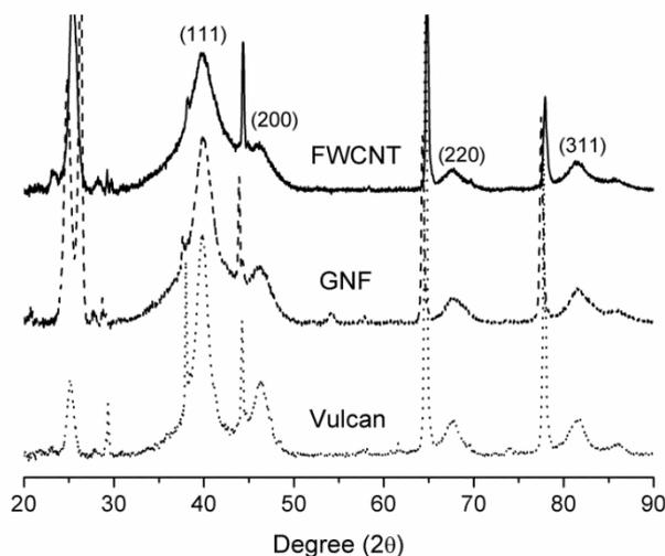
**Fig. 9. XRD pattern of the fresh anodes: PtRu supported on Vulcan, GNFs and FWCNTs.**
