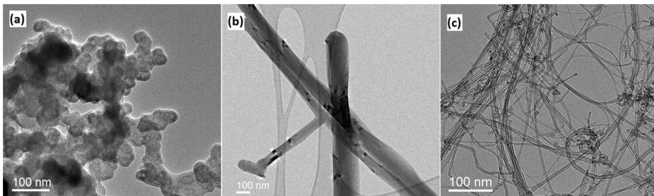
**Fig. 3. TEM images of the carbon supports: Vulcan (a), GNFs (b), FWCNTs (c).**
