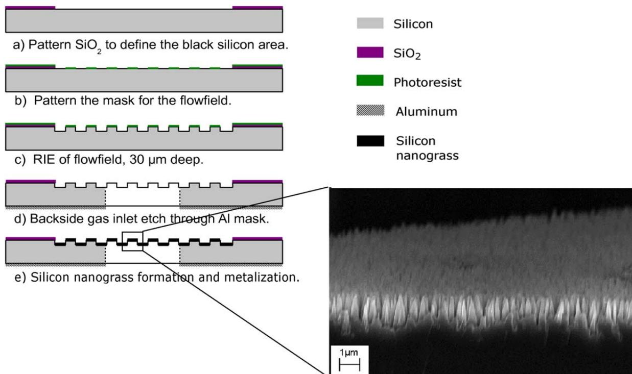
**Fig. 1. Main steps of microfabrication of a silicon chip. The inset shows nanograss formed on top of the flow fields.**
