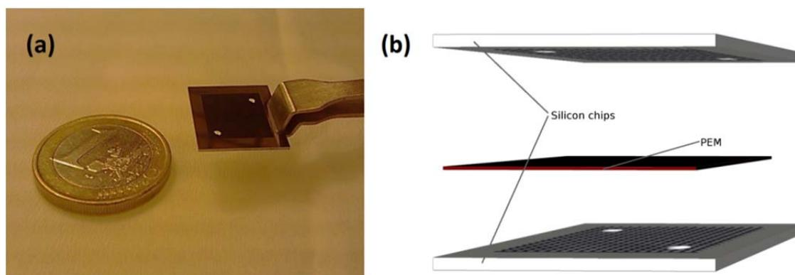
**Fig. 2. Photograph of a silicon chip (a) and Si-MFC construction by sandwiching the MEA between two silicon chips (b).**
