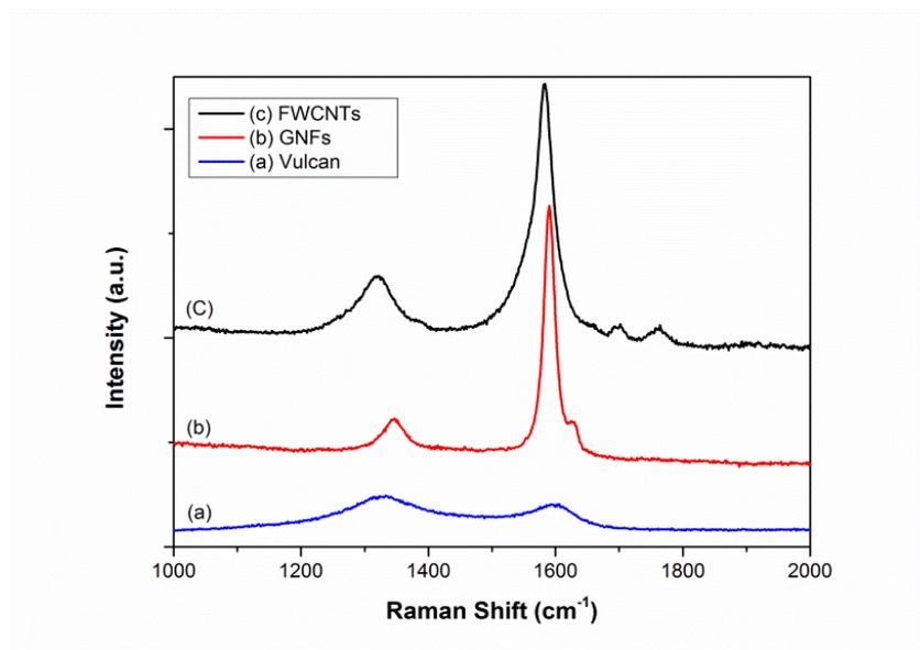
**Fig. 4. Raman spectra of pristine Vulcan, GNFs and FWCNTs.**
