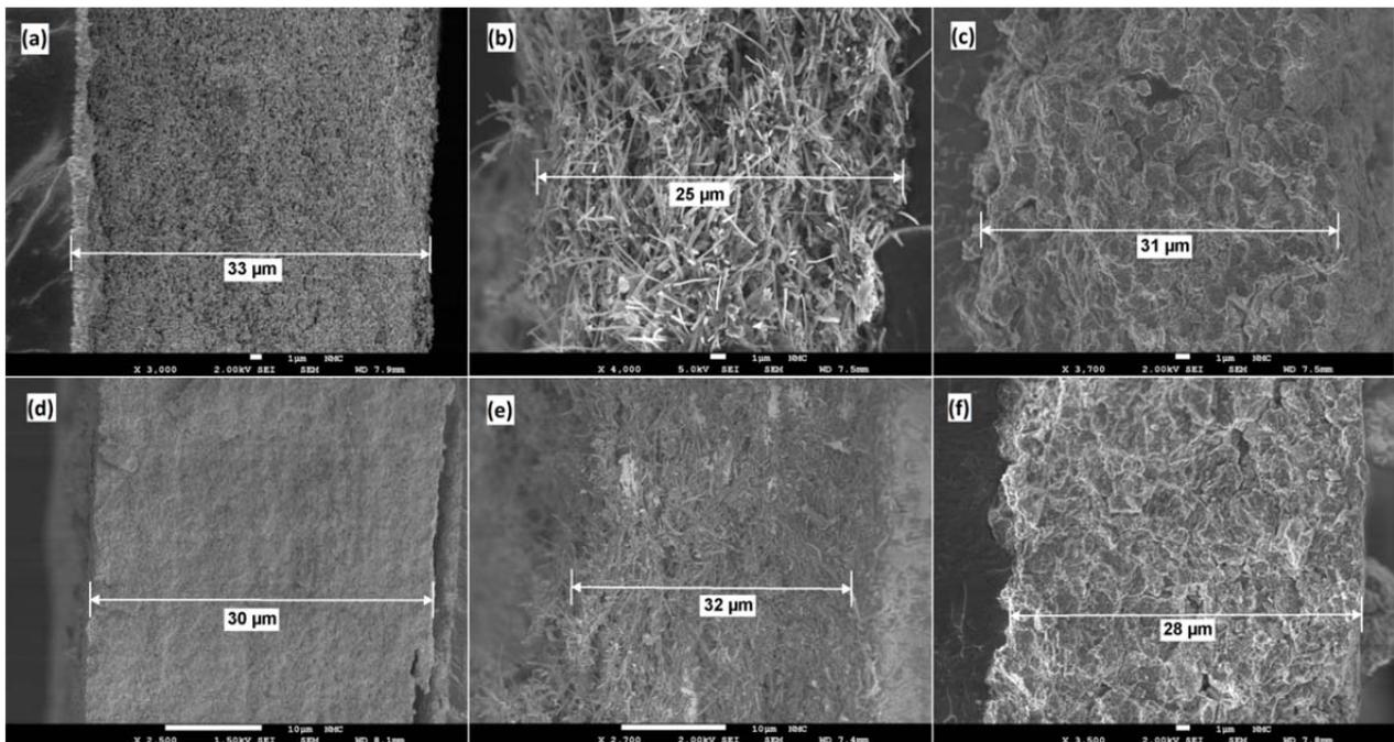
**Fig. 8. Cross-sectional SEM images of the anode layers before (a,b,c) and after (d,e,f) the durability tests; with PtRu catalysts on Vulcan (a,d), GNFs (b,e) and FWCNTs (c,f).**
