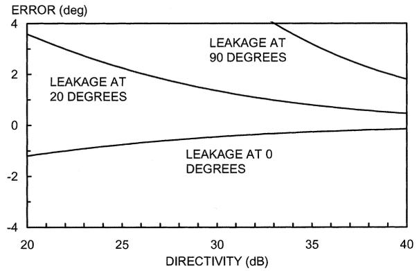
Fig. 5. Apparent phase error shown as a function of directivity with leakage phase offsets of  $0^\circ$ ,  $20^\circ$ , and  $90^\circ$ . Phase offsets between  $10^\circ$ – $20^\circ$  can normally be tolerated with coupler-related phase errors below  $1^\circ$ .
