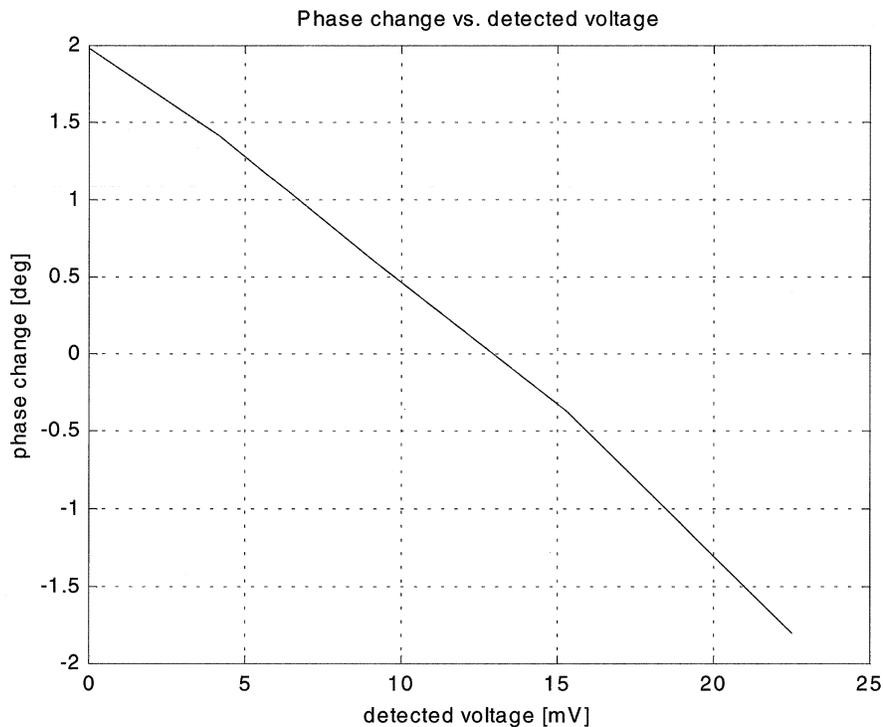
Fig. 2. Recorded phase detector output voltage versus phase change curve used for calibration. The phase detector coefficient is  $K_d = 6.4683\text{mV}/^\circ$ .
