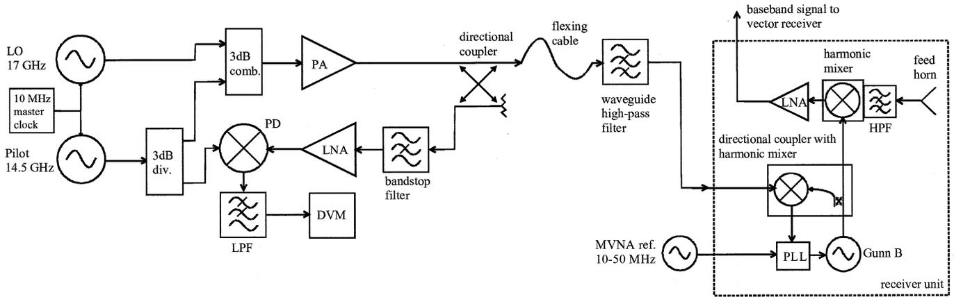
Fig. 1. Constructed real-time phase error measurement subsystem is shown with the submillimeter wave receiver. A lower frequency pilot signal is combined with the local oscillator signal, reflected back to the cable from the receiver, and coupled to the phase detector.
