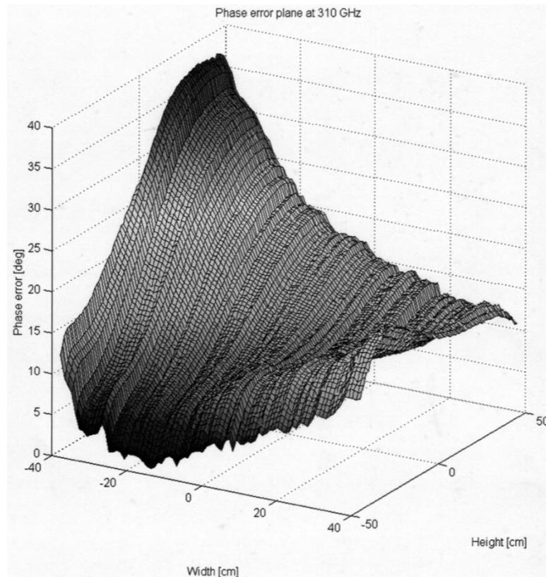
Fig. 6. Measured phase error plane across the largest scanning area of  $80 \times 90 \text{ cm}^2$ . The results are frequency-scaled to 310 GHz, and the maximum phase error is  $38^\circ$ .
