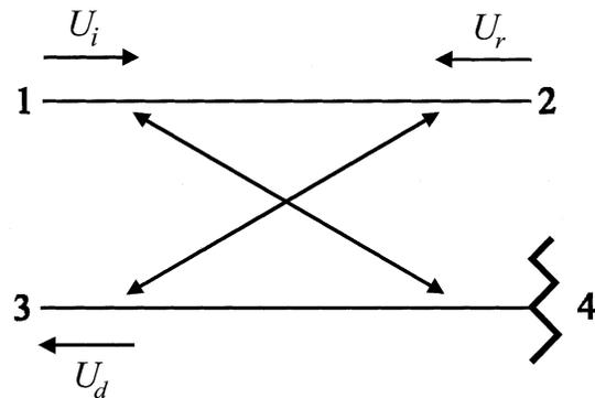
Fig. 3. The directional coupler can be thought as a three-port in which the unwanted coupling or leakage from port 1 to port 3 will cause phase performance degradation. The fourth port is assumed to be perfectly terminated. Here  $U_i$  is the incident signal,  $U_r$  the reflected signal, and  $U_d$  the raw sample to be fed to the phase detector.
