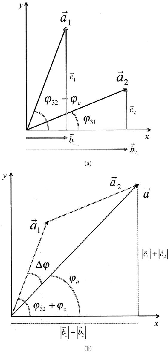
Fig. 4. (a) Definition of the used vectors for phase error calculation.  $\vec{a}_1$  is the wanted signal and  $\vec{a}_2$  the unwanted signal caused by the nonidealities in the directional coupler. (b) Definition of the sum vector with a phase angle of  $\varphi_a \cdot \varphi_{32} + \varphi_c$  is the phase angle of the wanted signal, and  $\Delta\varphi$  the phase bias caused by the unwanted signal.
