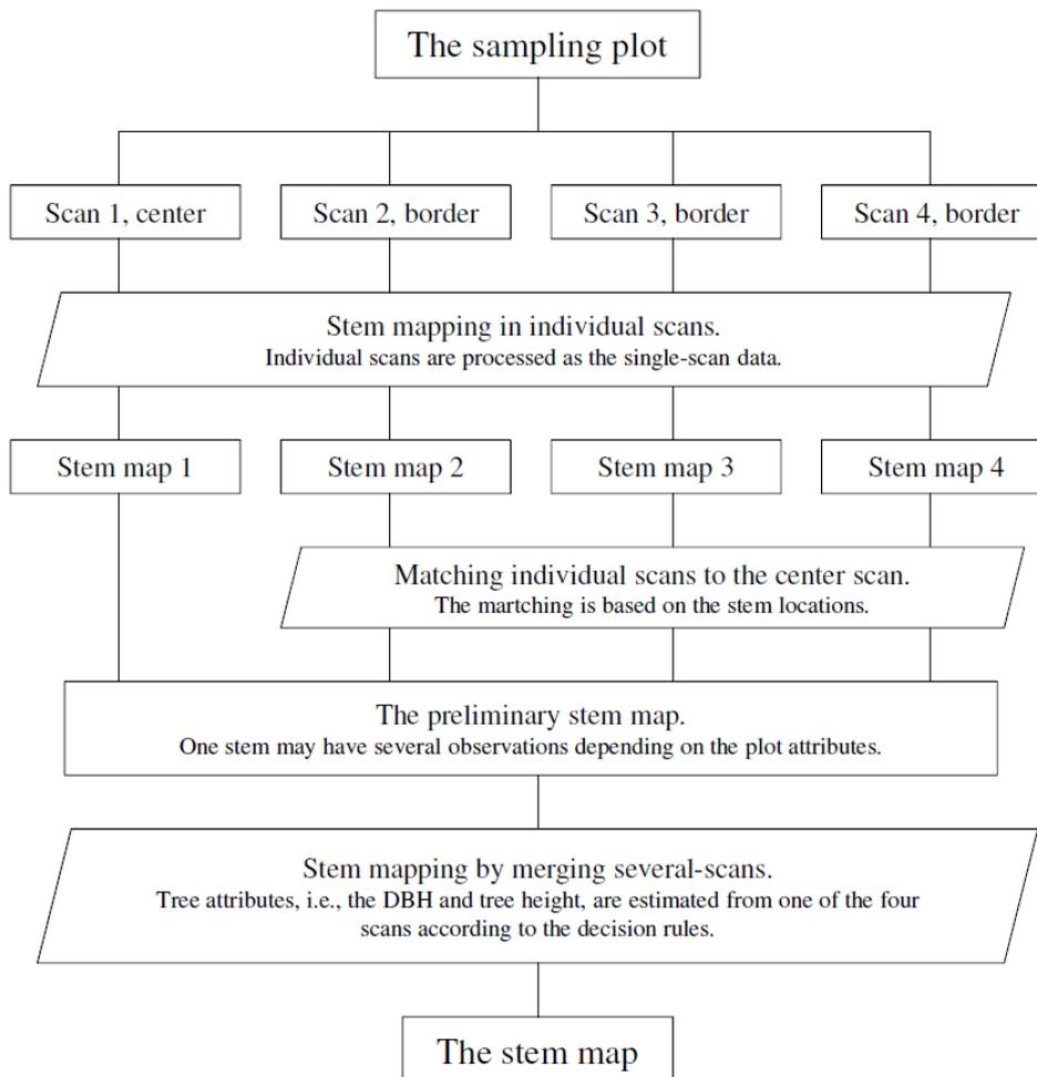
**Figure 6.** Conceptual diagram of the MSS method.
