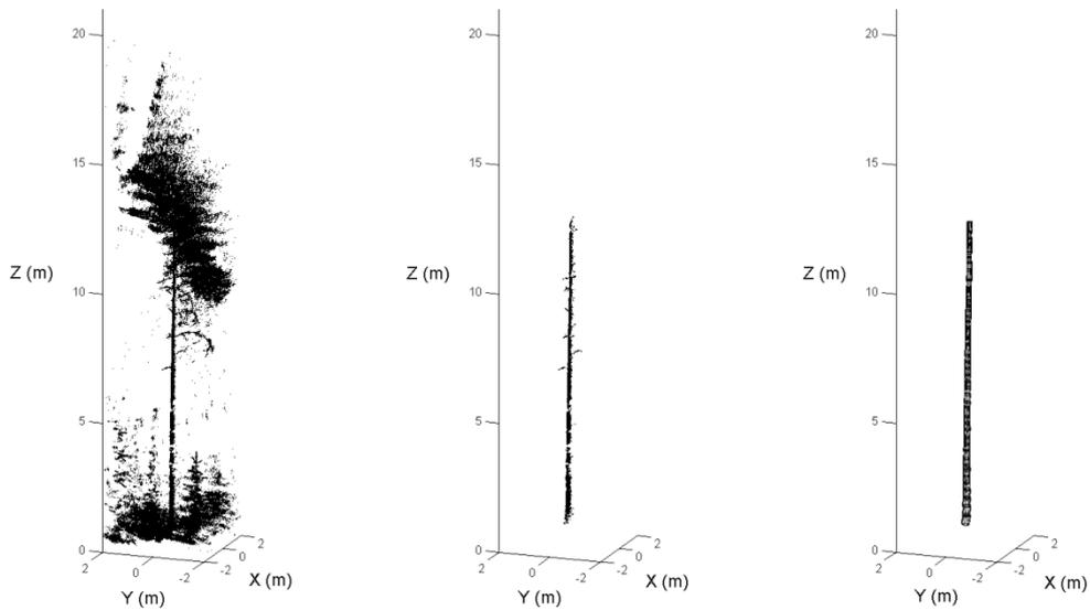
**Figure 5.** Automated stem reconstruction: (a) the original point cloud of a tree; (b) the detected stem points; and (c) the automatically reconstructed stem model.
