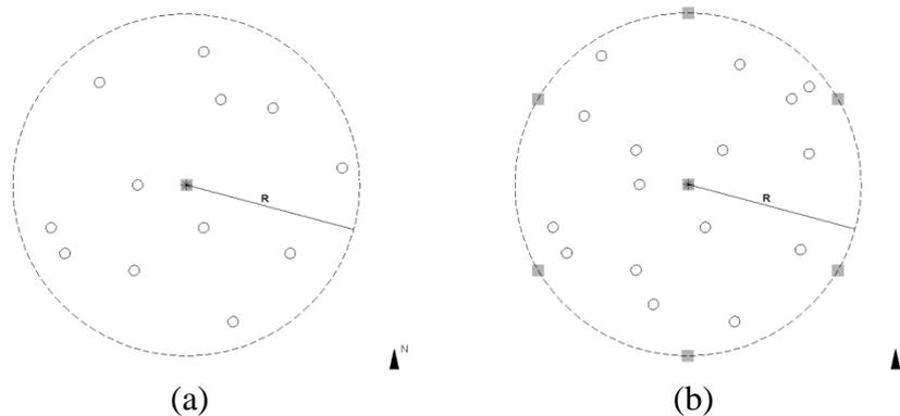
**Figure 2.** The scanning scenario of single-scan (a) and multi-scan (b) approaches. The sample plot is a circular area with radius  $R$ . The plot center is marked by an asterisk, and the positions of the trees are shown as solid circles. The gray squares indicate the scanning locations.
