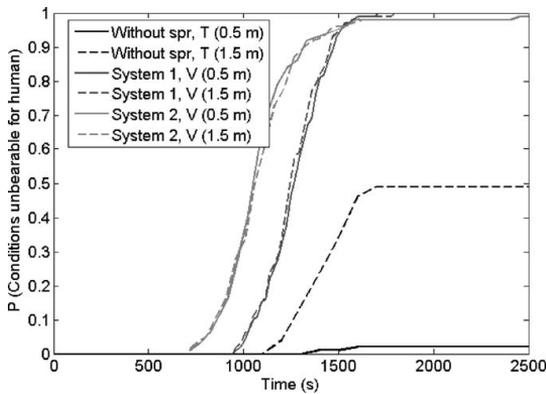
Fig. 10. Cumulative probability distributions for the time that the conditions for human get intolerable 7.5 m away from the ignition point. T, temperature criterion; V, visibility criterion.
