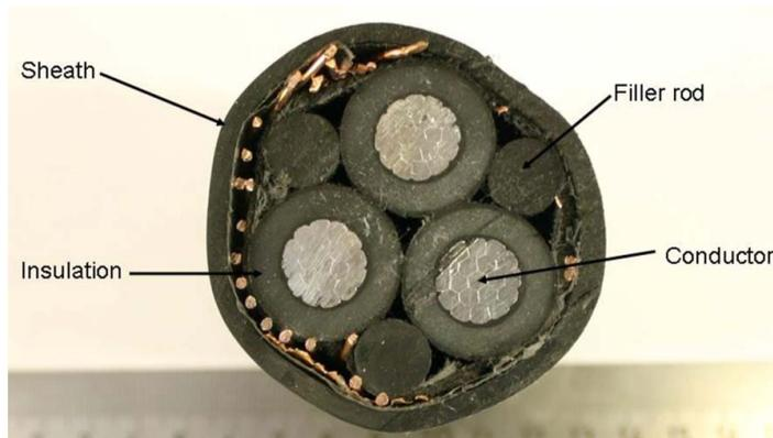
Fig. 3. Cross-section of the NOKIA AHXCMK 10 kV 3 × 95/70 mm<sup>2</sup> power cable.
