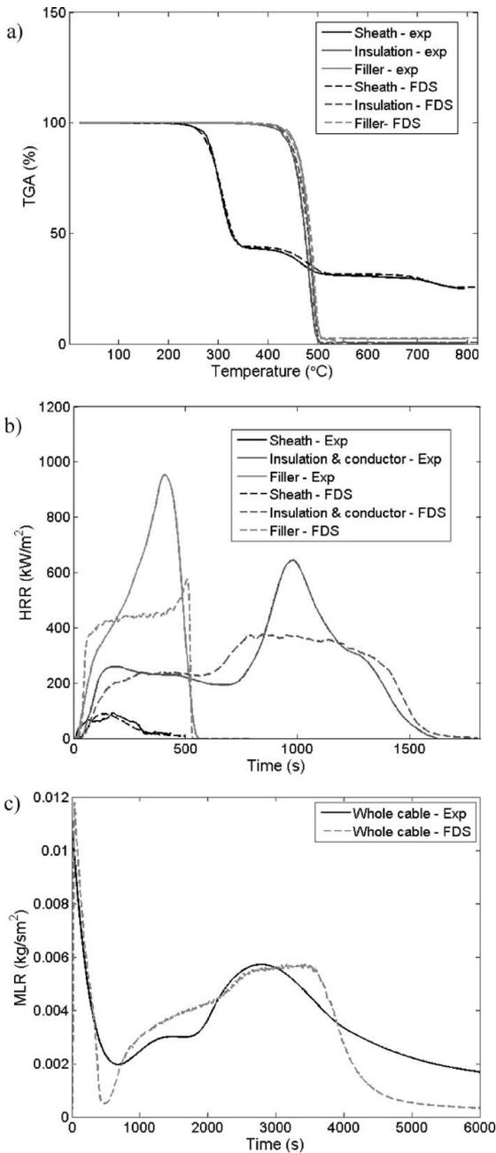
Fig. 4. Comparison of the experimental and simulated results. (a) TGA in nitrogen at heating rate 10 K/min. (b) Heat release rate of the components from cone calorimeter at 50 kW/m<sup>2</sup> heat flux. (c) Mass loss rate of the whole cable from cone calorimeter at 50 kW/m<sup>2</sup> heat flux.
