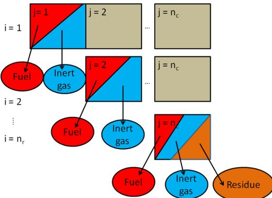
Figure 1. The reaction path assumption in Method 1.
