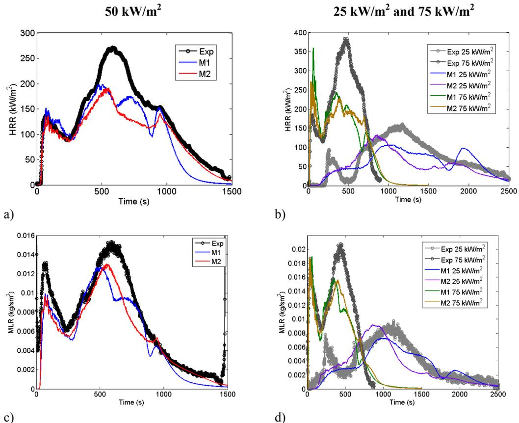
Figure 10. Cone calorimeter results for Method 1 and Method 2. a) Heat release rate at 50 kW/m<sup>2</sup>. b) Heat release rate at other heat fluxes. c) Mass loss rate at 50 kW/m<sup>2</sup>. d) Mass loss rate at other heat fluxes.
