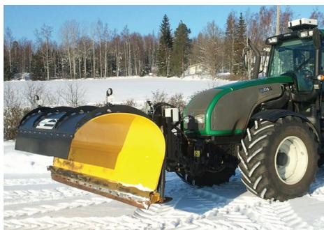
Figure 1. Snow plough was mounted into the front hitch of the tractor and the positioning devices was mounted on the roof of the tractor.
