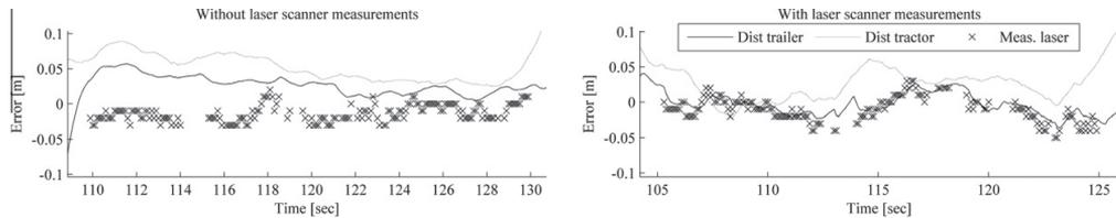
**Fig. 15.** Tracking errors in straight line following tests without (on the left) and with (on the right) laser scanner measurements in the Kalman-filter. Errors are measured by laser scanner and VRS-GPS.
