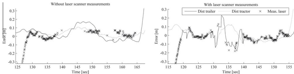
**Fig. 16.** Tracking errors in curved line following tests without (on the left) and with (on the right) laser scanner measurements in the Kalman-filter. The tractor went over the mark-furrow and the laser scanner was unable to measure the distance for the whole time.
