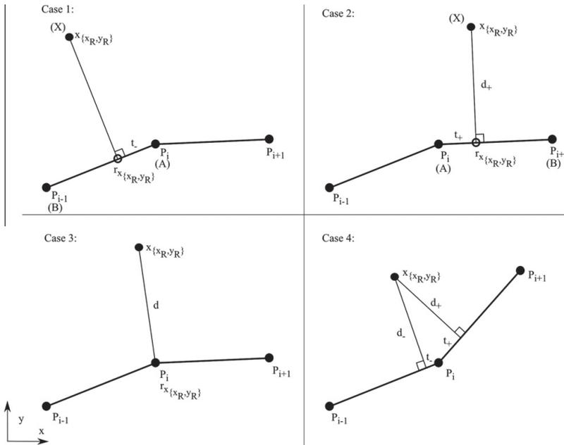
Fig. 4. Four different cases to calculate the trajectory point corresponding to the current state; Case 1: Position X is closest to the line  $P_{i-1} - P_i$ , Case 2: Position X is closest to the line  $P_i - P_{i+1}$ , Case 3: Position X is closest to path position  $P_i$  and Case 4: Inner curve.
