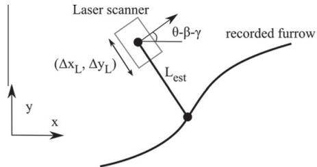
**Fig. 5.** Correcting the estimated position of the laser scanner using the laser scanner measurement and recorded furrow position. Notice, that  $L_{est}$  is not necessarily perpendicular to the furrow (as it is in the trajectory generation).
